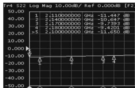
Figure 7 ·  $S_{22}$  plot in the 2100 MHz band (unchanged).
