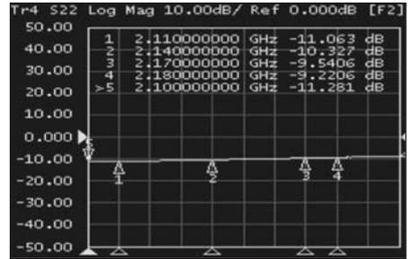
Figure 10 ·  $S_{22}$  plot after changing DC blocking capacitors.
