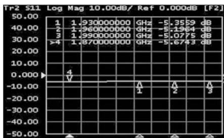
Figure 3 ·  $S_{11}$  plot in the 1900 MHz band.
