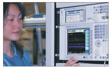
The Agilent MXG and MXA provide a compact test combination with the MXG providing the test signals and MXA performing the analysis. The MXA's on-board Windows XP PC controls the entire test process, including communications and any user-defined functions.
