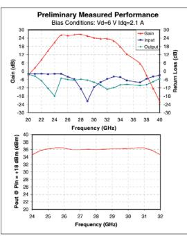
Plots of the TGA4905 gain and input/output return loss data (top); and power output over the band at +18 dBm input (bottom).
