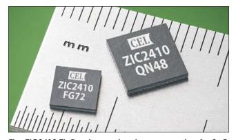
The ZIC2410 ZigBee transceiver is an example of a SoC device that intergrates multiple functions, inlcuding RF transceiver, power management, microcontroller and other support circuitry.
