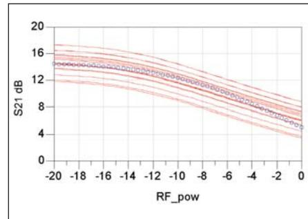
Figure 11 · Swept power gain measurement (dB) for the validation circuit compared with the model at 3.3V Vcc, 25°C and 2.4 GHz. Statistical analysis was performed on the inductors and capacitor to verify tolerance (10%) effects.
