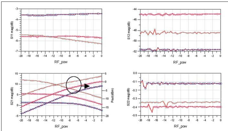
Figure 4 · Swept power  $S$ -parameter data on 4 mil Rogers 4350 for the 5116014H01 at 2.4V and  $25^{\circ}\text{C}$ , at 0.25 GHz, 0.75 GHz and 2.4 GHz. Red Line is model performance at 0.25 GHz, 0.75 GHz and 2.4 GHz; blue circles are measured data at 250 MHz; pink circles are measured data at 750 MHz, light blue circles are measured data at 2.4 GHz.
