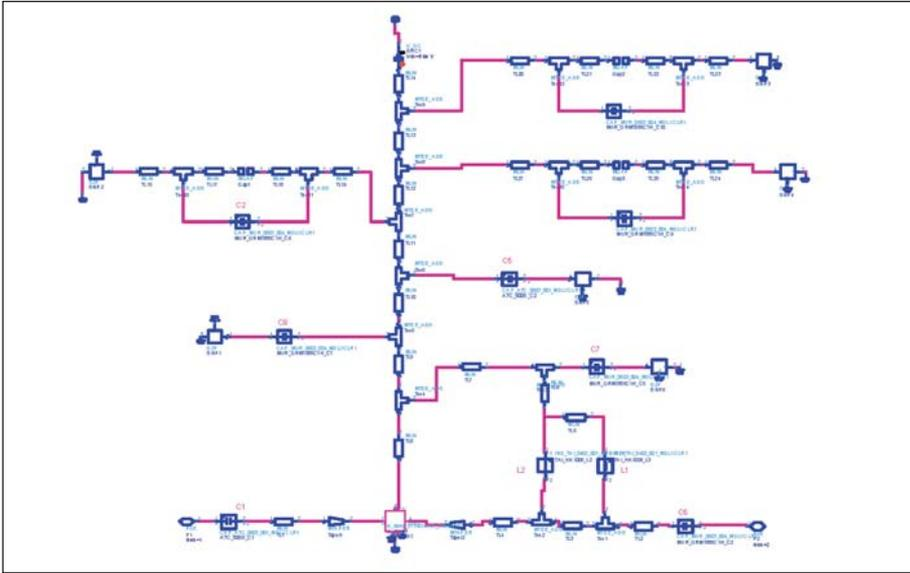
Figure 5 · Validation circuit design as represented in ADS 2006 using transmission line elements and Modelithics CLR components at 2.4 GHz.
