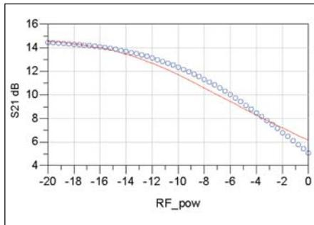
Figure 9 · Swept power gain (dB) for reference validation circuit compared with the model at 2.4V Vcc, 25°C and 2.4 GHz. Red line is model performance; blue circles are measurements on 16 mil Rogers 4003 substrate.
