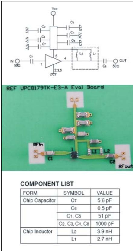
Figure 6 . The NEC UPC8179 2.4 GHz reference validation circuit design used in this work. The circuit was fabricated on a 16 mil Rogers 4003 board. Also shown is the manufacturers recommended component list.
