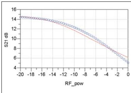
Figure 8 · Swept power gain (dB) for reference validation circuit (2.4 GHz) for NEC UPC8179 amplifier on 16 mil Rogers 4003 compared with the model at 2.4V Vcc, 25°C. Red line is model performance; blue circles are measurements.
