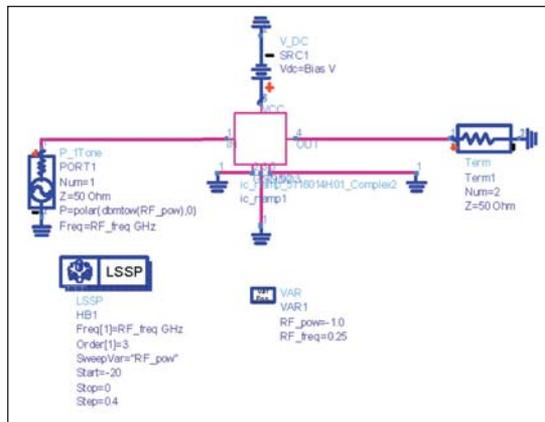
Figure 2 . ADS Test Bench for large signal *S*-parameters using the P2D Data file format.
