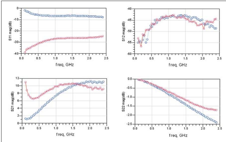
Figure 3 · Simulated small-signal  $S$ -parameter data on 4 mil Rogers 4350 and 16 mil Rogers 4003 compared to the model at 3.3V,  $-40^{\circ}\text{C}$ . Blue circles are measurements on 4 mil Rogers 4350 substrate; light blue line is model performance for 4 mil Rogers 4350; pink circles are measurements on 16 mil Rogers 4003; red line is model performance for 16 mil Rogers 4003.
