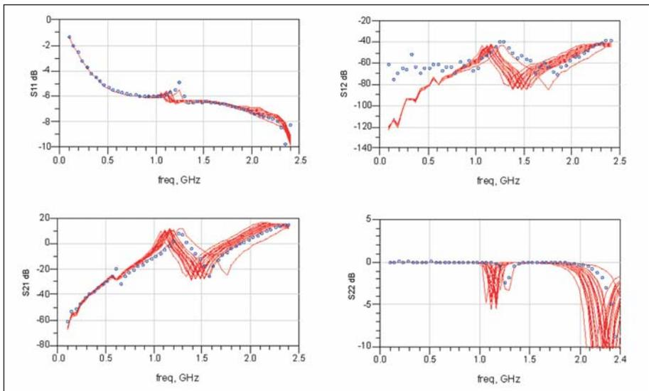
Figure 10 · S-parameter data for reference validation circuit compared with the model at 3.3V Vcc, 25°C. Statistical analysis has been performed on the Taiyo Yuden inductors (2.7 nH and 3.9 nH) and Murata capacitor (5.6 pF) to analyze tolerance (10%) effects.
