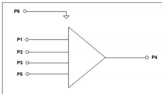
Figure 1 . NEC UPC8179TK-E2-A amplifier model topology. Pins P2, P3, and P5 are not used in this particular part’s model.
