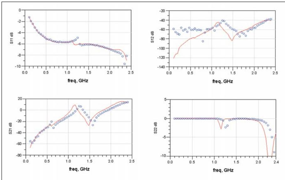
Figure 7 · S-parameter data for the validation circuit for NEC UPC8179 amplifier on 16 mil Rogers 4003 compared with the model at 2.4V Vcc, 25°C. Red line is model performance; blue circles are measurements using 16 mil Rogers 4003 substrate.
