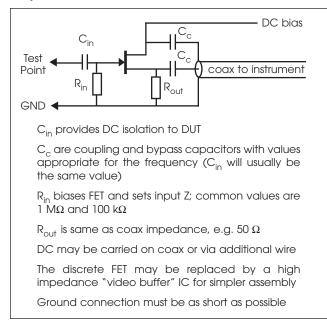
Of course, a lab-built probe will not have accurate calibration, and may not have the bandwidth of a good commercial probe. They are most valuable when approximate measurements are sufficient.
