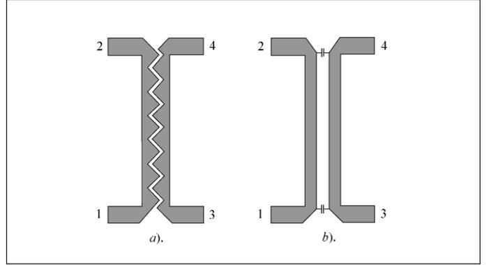
Figure 42 · Coupled-line directional couplers with compensation for directivity vs. frequency.
