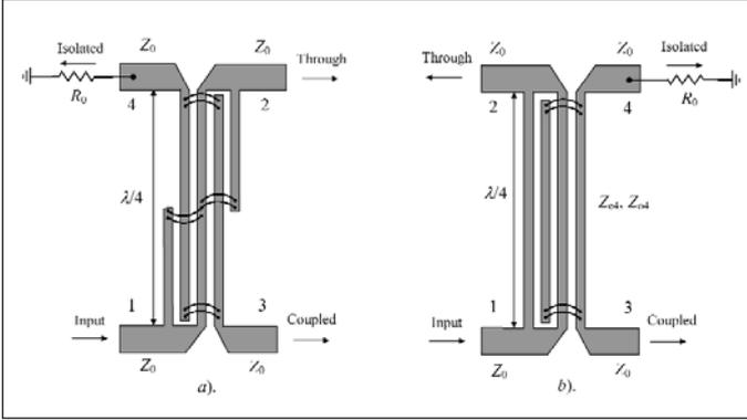
Figure 41 · Lange directional couplers: (a) original interdigital configuration, and (b) “unfolded” version.
