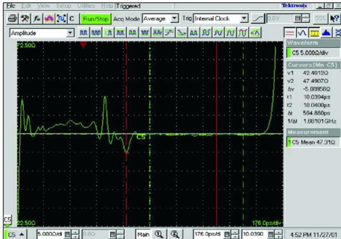
Figure 9 · This measurement window includes the transition from the CSA RF module to the microstrip test board, as well as the coaxial-to-microstrip launch transition from the SMA connector.
