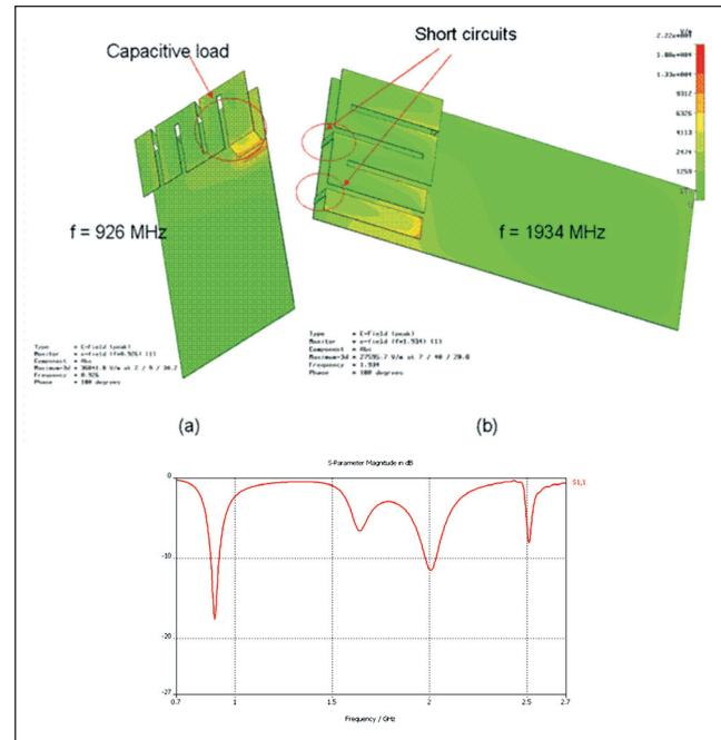
This dual-band patch antenna is an example of a structure developed for a specific application, using electromagnetic simulation and analysis software. (Image courtesy CST)
