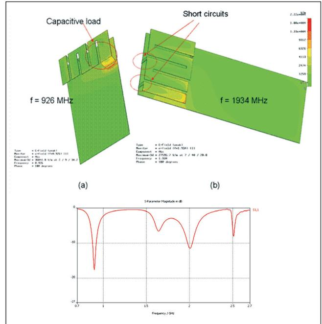
This dual-band patch antenna is an example of a structure developed for a specific application, using electromagnetic simulation and analysis software. (Image courtesy CST)
