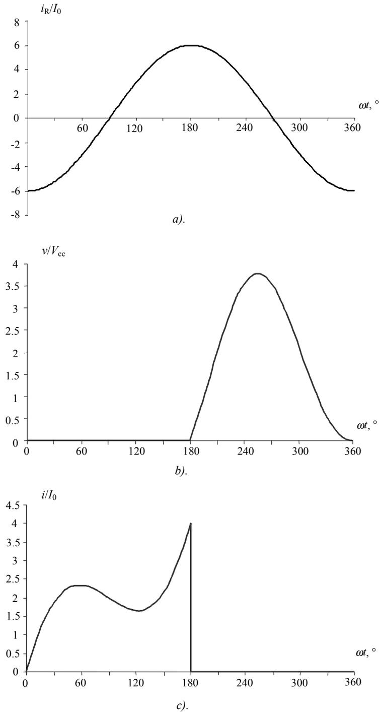
Fig. 5. Normalized (a) load current and collector (b) voltage and (c) current waveforms for idealized optimum even harmonic Class E
