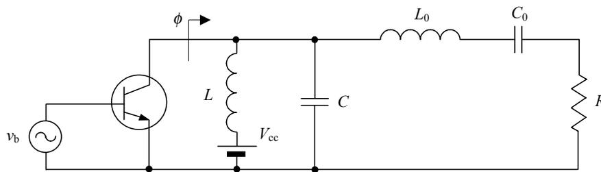
Fig. 6. Equivalent circuit of the parallel-circuit Class E power amplifier
