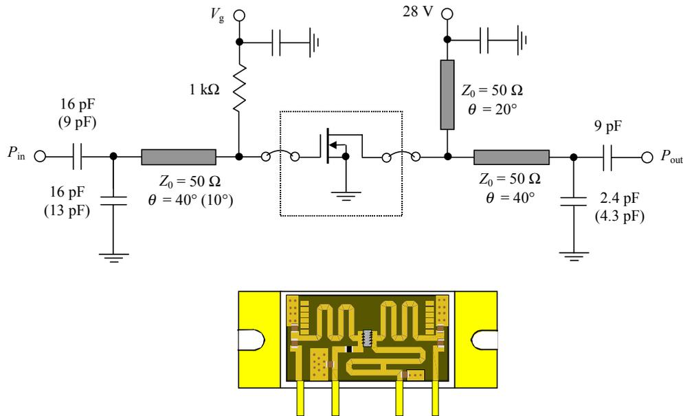
Fig. 12. Circuit schematic and module design of single-stage 500 MHz parallel-circuit Class E high-voltage LDMOSFET power amplifier
