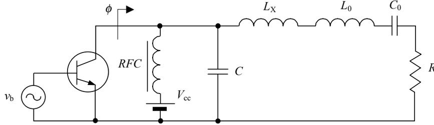
Fig. 2. Equivalent circuit of the Class E power amplifier with shunt capacitance
