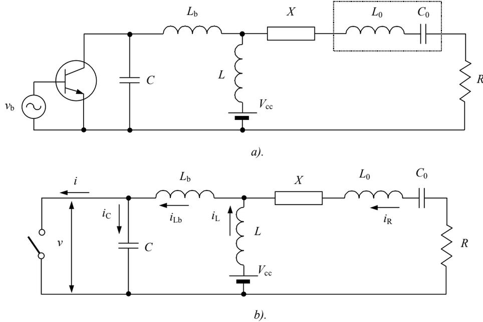
Fig. 1. Equivalent circuits of the Class E power amplifiers with generalized load network
