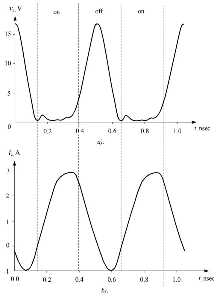
Fig. 14. Simulated (a) collector voltage and (b) current waveforms of transmission-line parallel-circuit Class E low-voltage InGaP/GaAs HBT power amplifier
