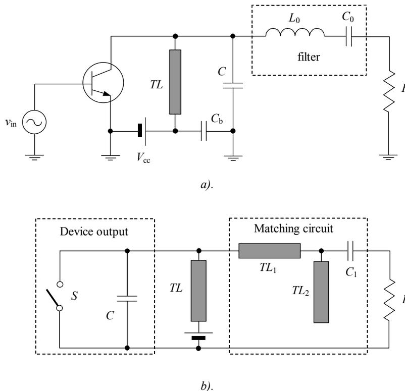
Fig. 10. Equivalent circuits of transmission-line parallel-circuit Class E power amplifier
