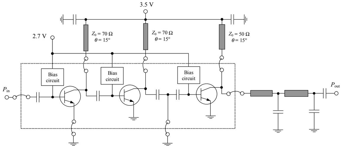
Fig. 13. Circuit schematic of high-efficiency low voltage three-stage dual-band DCS1800/PCS1900 power amplifier
