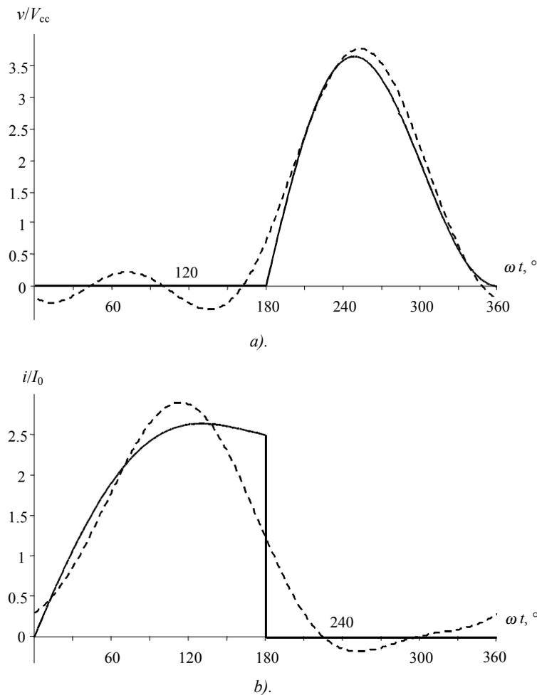
Fig. 9. Two-harmonic approximation to parallel-circuit Class E
