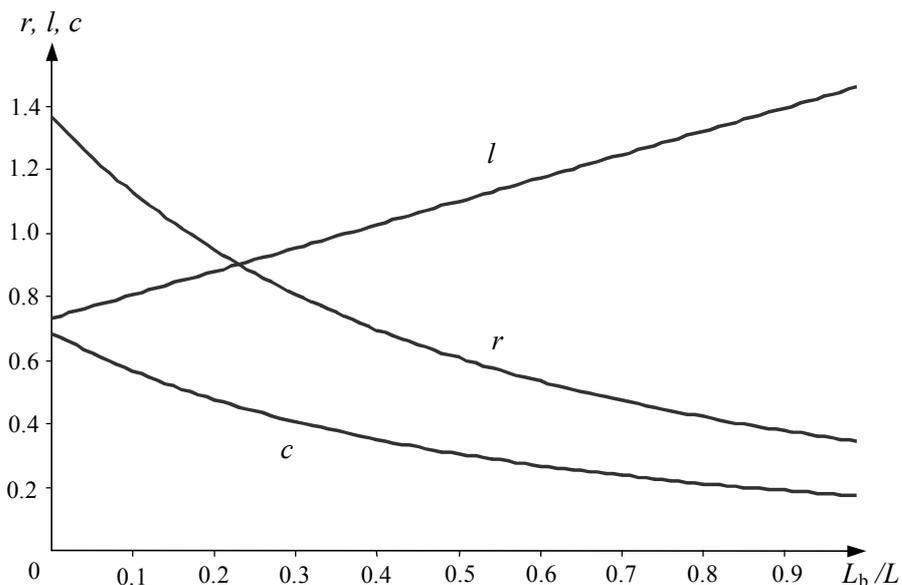
Fig. 8. Normalized optimum load network parameters versus normalized bondwire inductance  $L_b/L$  for parallel-circuit Class E
