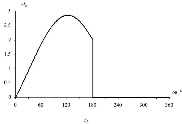
Fig. 3. Normalized (a) load current and collector (b) voltage and (c) current waveforms for idealized optimum Class E with shunt capacitance
