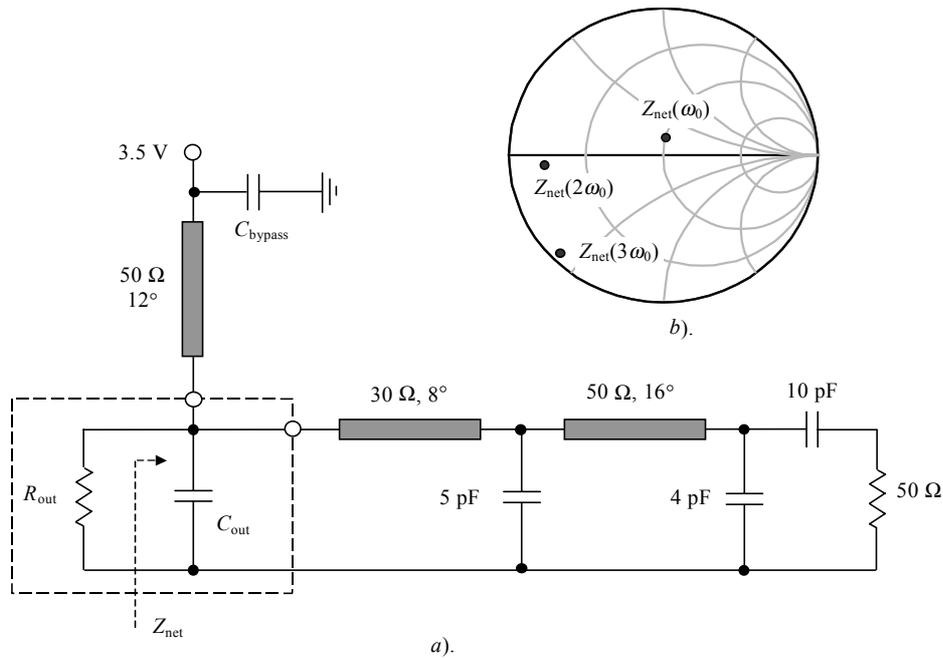
Fig. 11. Output load network of transmission-line parallel-circuit Class E power amplifier for handset application
