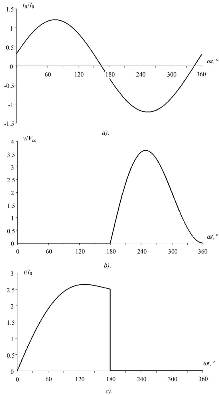
Fig. 7. Normalized (a) load current and collector (b) voltage and (c) current waveforms for idealized optimum parallel-circuit Class E
