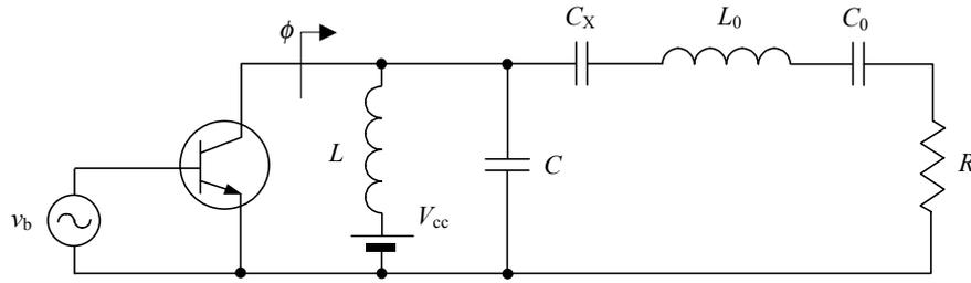
Fig. 4. Equivalent circuit of the even harmonic Class E power amplifier
