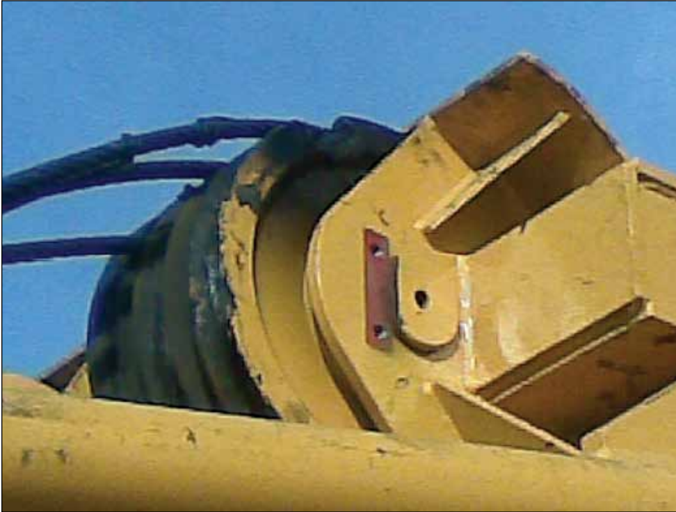
Figure 2 • Detail of the burnt pulley, showing the damage to the sheave and cables.
