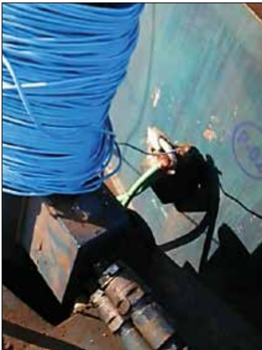
Figure 9: (a) The implemented coil and (b) the wire connecting the hook to the coil.
