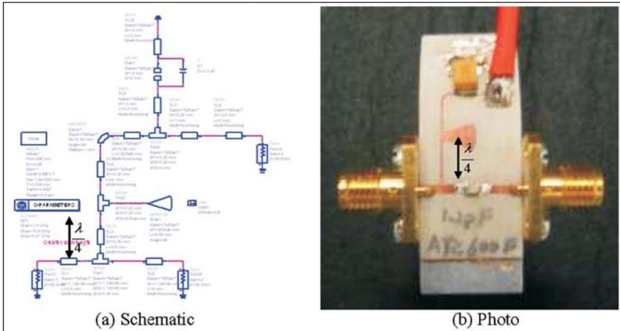
Figure 1 · The bias network consists of a quarter-wavelength radial stub and a tantalum capacitor.
