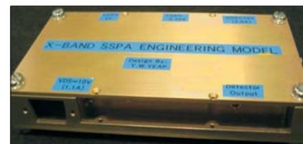
Figure 9 · Outer view of the optimized HPA module.
