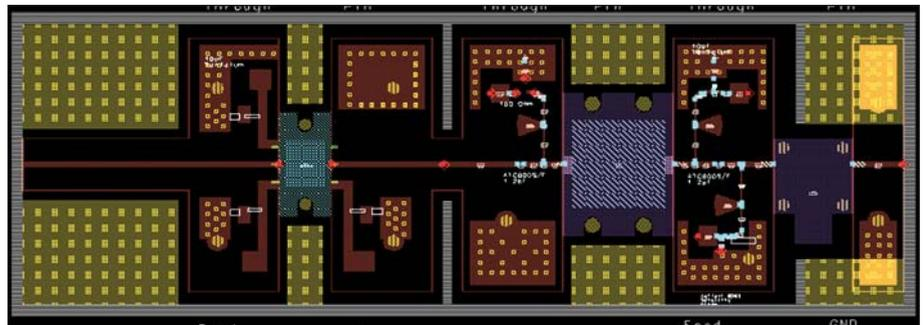
Figure 5 · PCB layout of HPA module.
