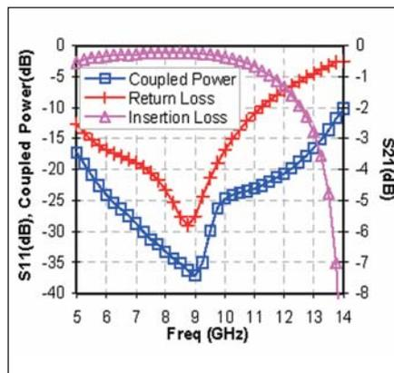
Figure 3 · Measured insertion loss, return loss and coupled power of the X-band power divider.
