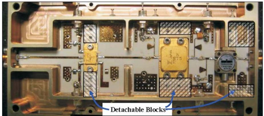
Figure 6 · Inner view of HPA module developed.
