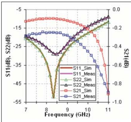
Figure 2 · Simulated and measured S-parameters of the DC bias network.
