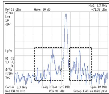
Figure 8 · Spectrum plot showing the output carrier with spurious caused by RF in the DC supply.
