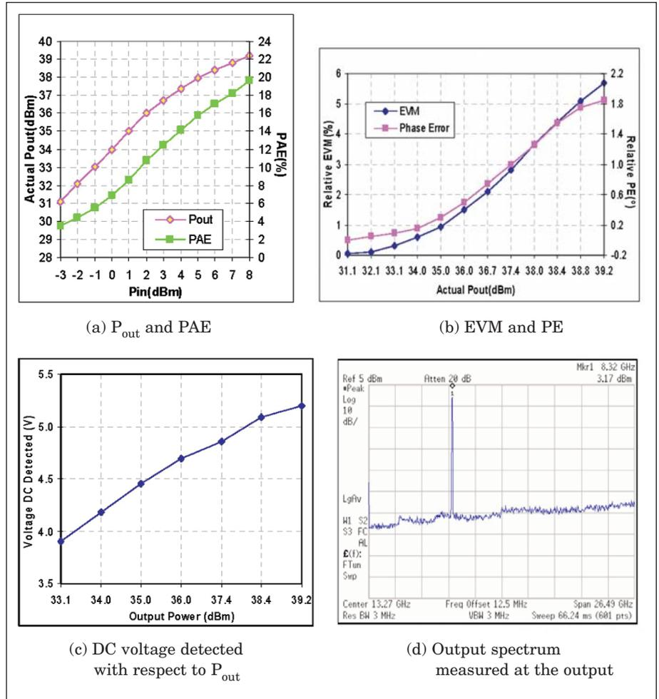
Figure 10 · Performance of the optimized HPA module.
