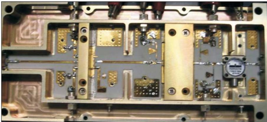
Figure 7 · Removing cavity resonance using aluminium blocks that extend over the HPA devices.
