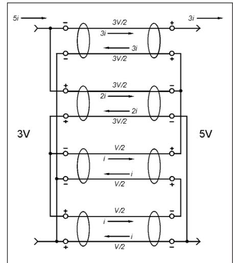
Figure 16 · Order-4 TLT having a 3:5 (1:2.78 impedance) ratio.
