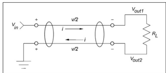
Figure 9 · Order-1 TLT used as a 1:1 choke balun.
