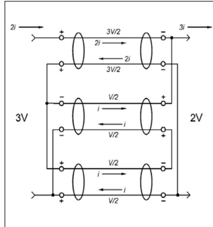
Figure 15 · Order-3 TLT having a 3:2 voltage (2.25:1 impedance) ratio.
