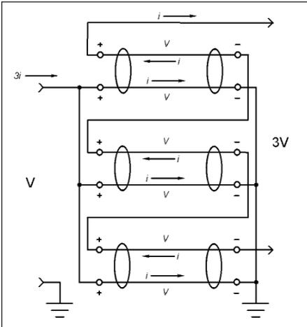
Figure 13 · Order-3 TLT used as a 3:1 current (1:9 impedance) balun.
