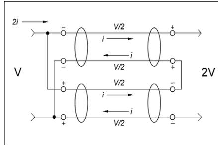
Figure 14 · The Guanella 1:4 impedance ratio TLT, which uses two lines.
