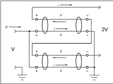
Figure 12 · Order-2 TLT used as a 2:1 current (1:4 impedance) balun.
