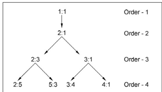
Figure 8 · Voltage transformation ratios of the first four orders of TLTs (from Rotholz (7)).
