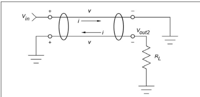
Figure 10 · Order-1 TLT used as a 1:1 phase inverter.
