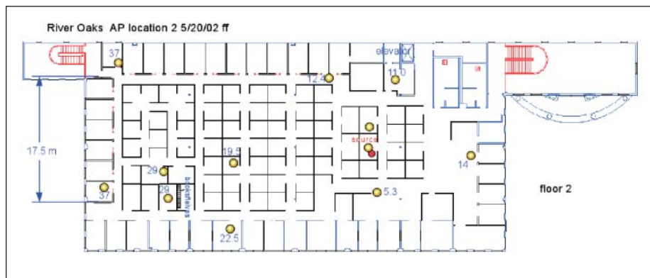
Figure 2 · Floor plan showing the measurement locations of additional 5.2 GHz points; access point site #2.
