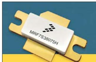
Samples of the initial 3.5 GHz LDMOS device are available now. The MRF7S38075H is a 75 watt  $P_{1dB}$
