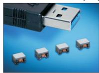
frequency improvement compared to previous products is achieved through the CM01S600's use of an extremely precise wire-wound structure.
