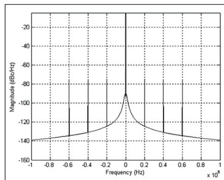
Figure 7 · PLL output spectrum.
