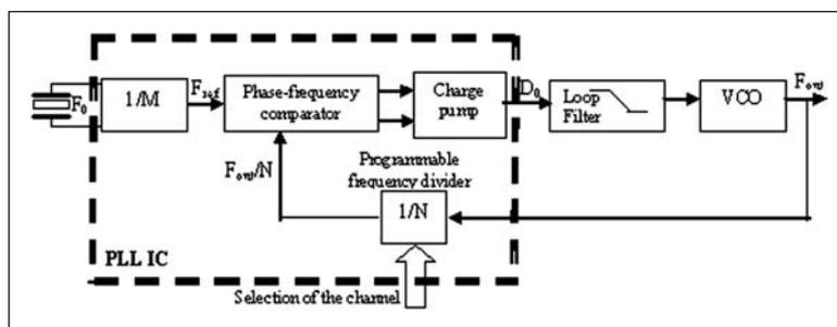
Figure 1 · Block diagram of the designed frequency synthesizer.
