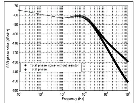
Figure 5 · SSB phase noise with and without resistor noise
