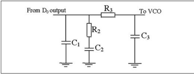
Figure 2 · Loop filter circuit.
