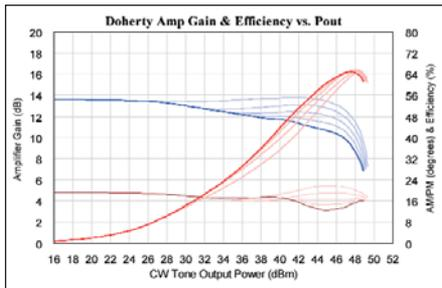
Figure 4 · Simulated gain and efficiency versus CW output power, for different gate bias voltages for the peaking amplifier (1.8/4.7 dB input coupler). The dark trace is for  $V_{gs} = -5$  volts. Voltage steps are 0.5 V.
