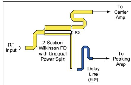
**Figure 2 · Schematic of an unequal power divider for Doherty application.**
