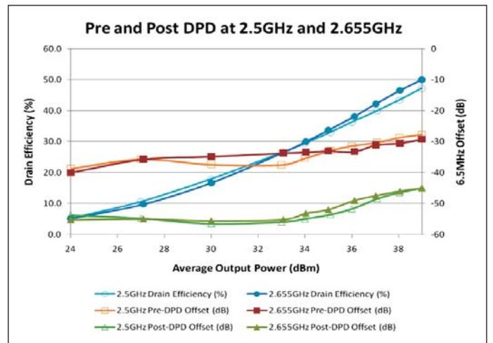
Figure 16 · Doherty amplifier spectral mask vs. average output power, with and without DPD correction (F = 2.5, 2.655 GHz, V<sub>supply</sub> = +28 V).
