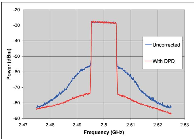
Figure 15 · Doherty amplifier spectral mask, with and without DPD correction (F = 2.5 GHz, P<sub>ave</sub> = 8 watts, V<sub>supply</sub> = +28 V, I = 600 mA, 48% DC-RF efficiency).
