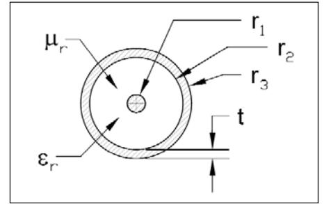
Figure 5 · Coaxial transmission line.
