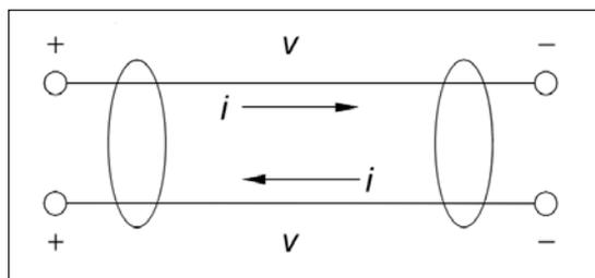
Figure 1 · Transmission line in transverse (TEM) mode.
