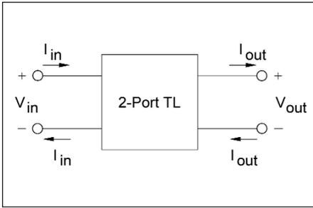
Figure 3 · TEM transmission line as 2-port ABCD element.
