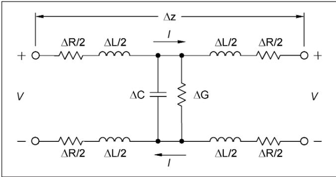
Figure 2 · Incremental model of TEM transmission line.
