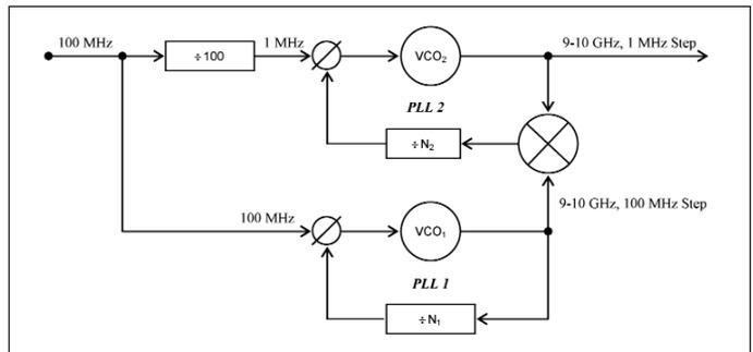
Figure 47 · Dual-loop synthesizer example.
