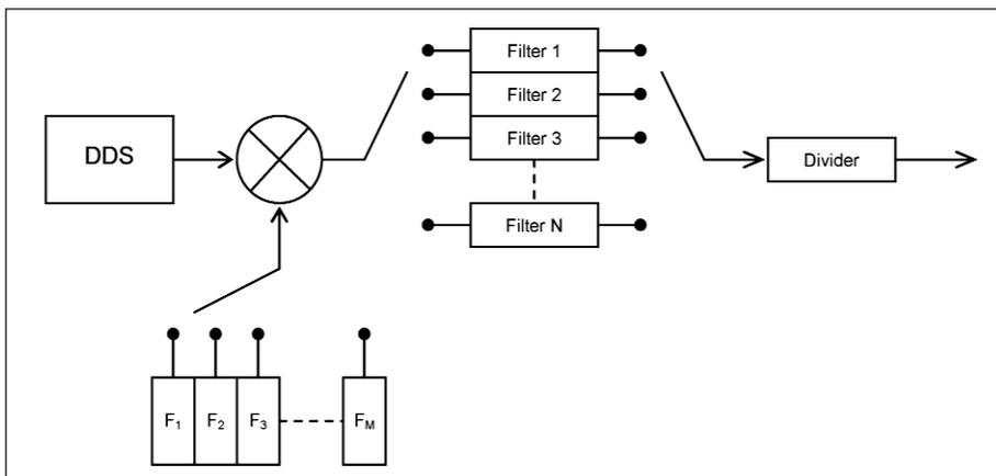
Figure 42 · DDS bandwidth extension.
