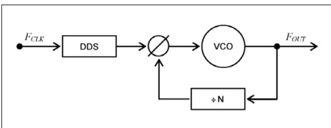
Figure 39 · Using DDS as a reference.
