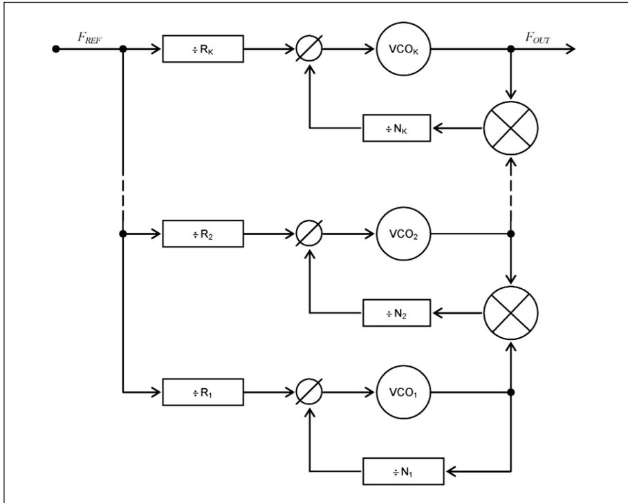
Figure 48 · Multiloop synthesizer concept.
