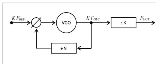
Figure 37 · A simple way to improve single-loop PLL performance.
