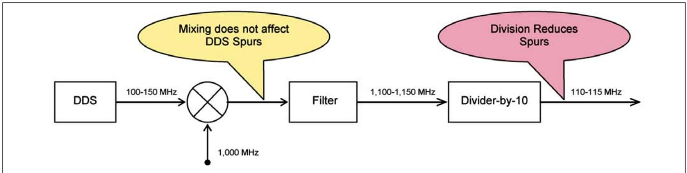
Figure 41 · DDS spur reduction.
