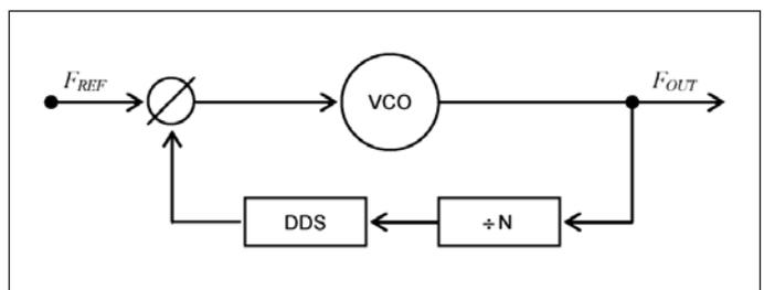
Figure 40 · Using DDS as a fractional divider.
