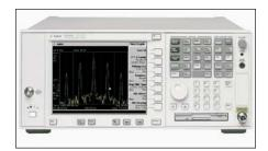
Benchtop instruments like the Agilent Technologies PSA series offer laboratory performance plus a wide range of options and analysis capabilities.
