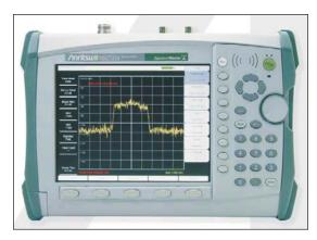
Handheld portable spectrum analyzers with high performance, like this Anritsu MS2721A, are among the recent developments by instrument manufacturers.
