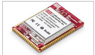
Figure 2 · The MC13224 from Freescale<sup>™</sup> is a single-chip platform-in-package (PiP) transceiver that integrates a 32-bit ARM7 processor. This powerful MCU, combined with generous on-chip memory, allows designers to run complex applications without the need for peripheral processing devices. CEL packages the MC13224 in its FreeStar PRO radio module. FCC, IC and CE certified, it eliminates the costly and time-consuming certification process.
