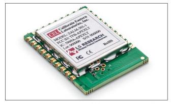
Figure 1 · A variety of ZigBee/802.15.4 transceiver ICs are available. Ember<sup>™</sup> combines an RF transceiver with a flash-based co-processor in its EM260 chip. The EM260 stores the ZigBee stack in its flash memory, but takes commands from the processor that is resident in the enduser system. CEL's Apex LT combines the EM260 with a 100 mW power amplifier in an easy-to-use, drop-in radio module. FCC, IC and CE certified, these modules are ideal for designers looking for fast time-to-market.
