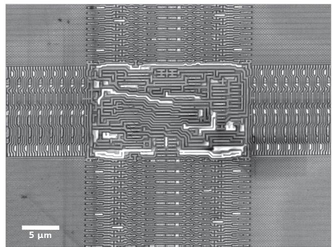
**Fig. 1.** Passive voltage contrast on an integrated circuit.
