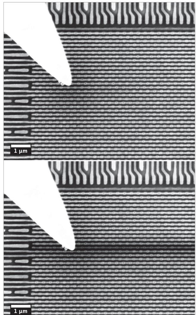
**Fig 3.** Selective biasing of a single, 100 nm wide interconnect line. Top: Before tip contact. Bottom: Contacting the line.
