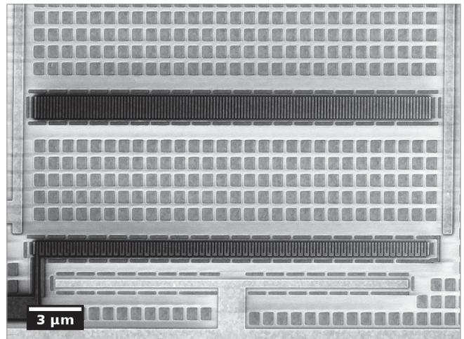
**Fig. 5.** Closed circuit biasing of contact chain structures using two tips (Tips not show in the image). The voltage drop along the chain structures becomes visible as a gradual decrease of voltage contrast.
