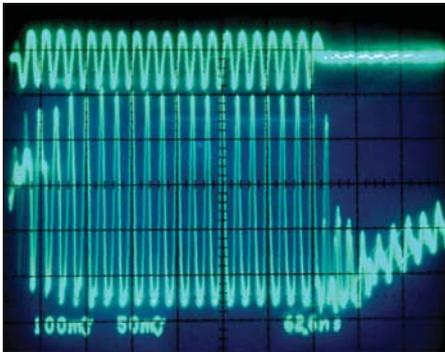
Figure 5 · 400 ns pulsed output waveform of the generator in Fig. 4 (upper trace), and the waveform after one stage of the zero group delay filter (lower trace).
