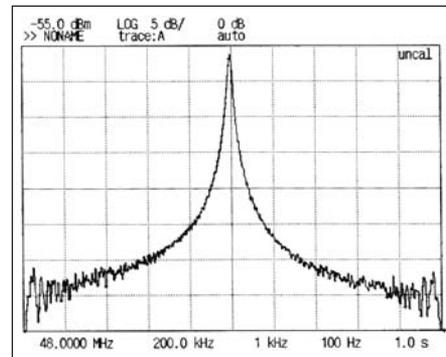
**Figure 3** · Swept bandpass of one stage of the half lattice or bridge filter at 48 MHz. The filter is balance tuned with equal slopes on both sides for pulse systems. These filters can be cascaded to increase the shoulder reduction. In the following examples, two or more stages are cascaded with a total sideband reduction of 40 dB. The 3 dB noise bandwidth of this filter at 48 MHz is approximately 500 Hz.
