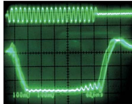
Figure 7 · The detected waveform of the 400 ns pulse using a synchronous detector. The rectangular waveform of the baseband pulse has been preserved.
