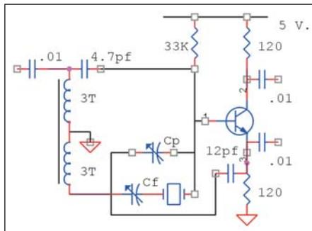
**Figure 2** · Schematic of the “half lattice” or “bridge derived” narrow band filter. This filter has near zero group delay and a very narrow noise bandwidth. The capacitor  $C_p$  must be very small (1- 2 pF).  $C_f$  determines the frequency of the filter. It may require as much as 40-50 pF to tune the filter to the nominal center frequency. Tune  $C_p$  first to obtain the swept spectrum seen in Figure 3, then adjust the frequency with  $C_f$ .
