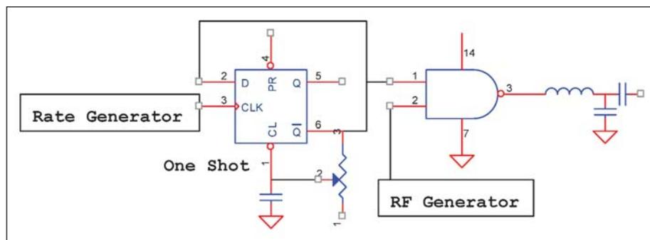
**Figure 4** · RF Pulse generator used for these experimentals.
