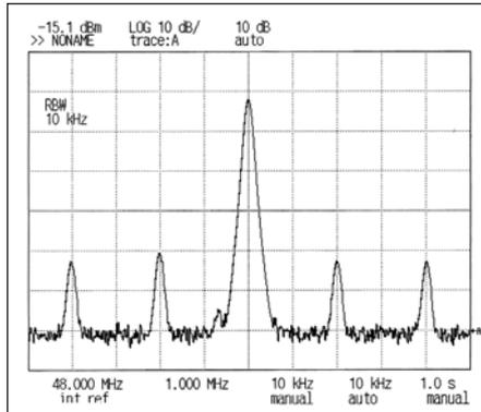
Figure 6 · The spectrum after two stages of the near zero group delay filter, showing the sidebands reduced by 40 dB. These sidebands are too weak to have an effect on the detected pulse signal.
