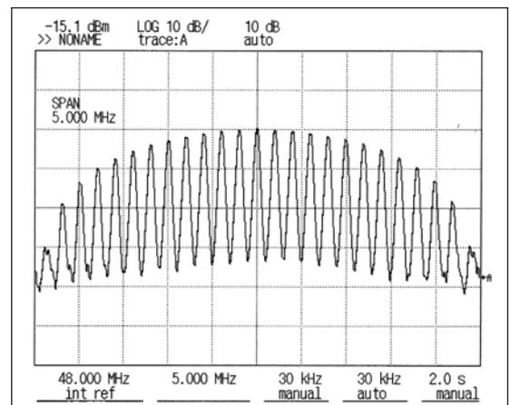
Figure 1 - Sinx/x Pulse spectrum for a pulse width of 400 nanoseconds with a repetition rate of 200 kHz. Most pulse systems would not use a rate this high.
