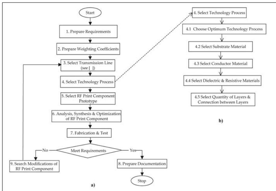
Figure 1 · Passive integrated circuit tradeoff analysis flow chart.
