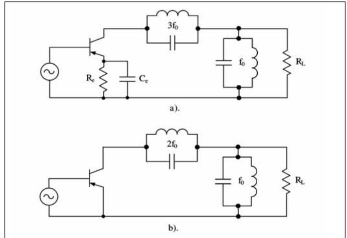
Figure 8 · Bi-harmonic bipolar-transistor power amplifiers.
