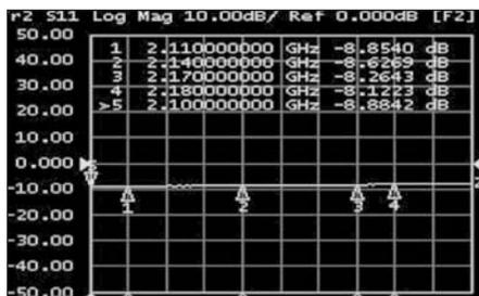
Figure 17 · S<sub>11</sub> plot after inductance correction and final tuning.
