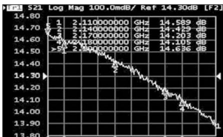
Figure 16 · S<sub>21</sub> plot after inductance correction and final tuning.
