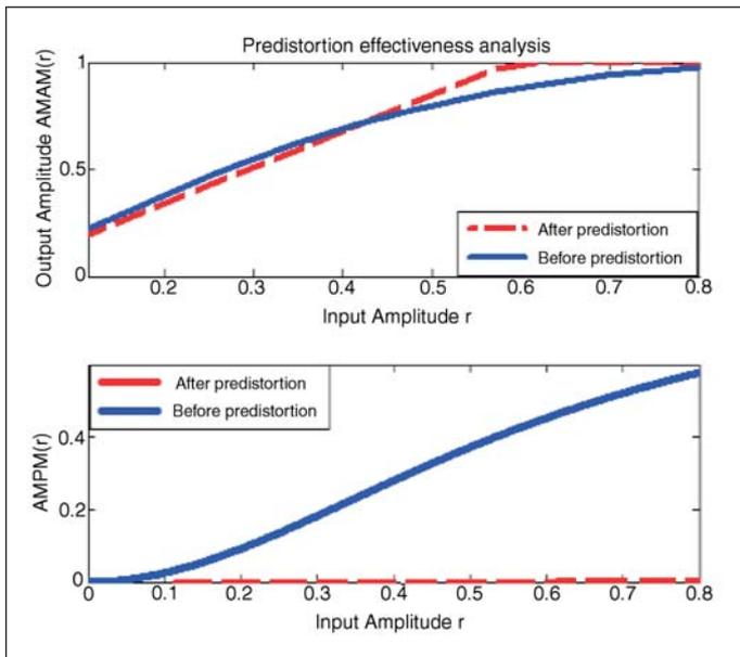
**Figure 8 · I/O transfer characteristic after predistortion.**
