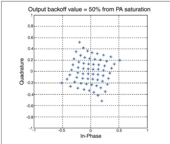
**Figure 6 · Signal representation for the predistorted constellation.**
