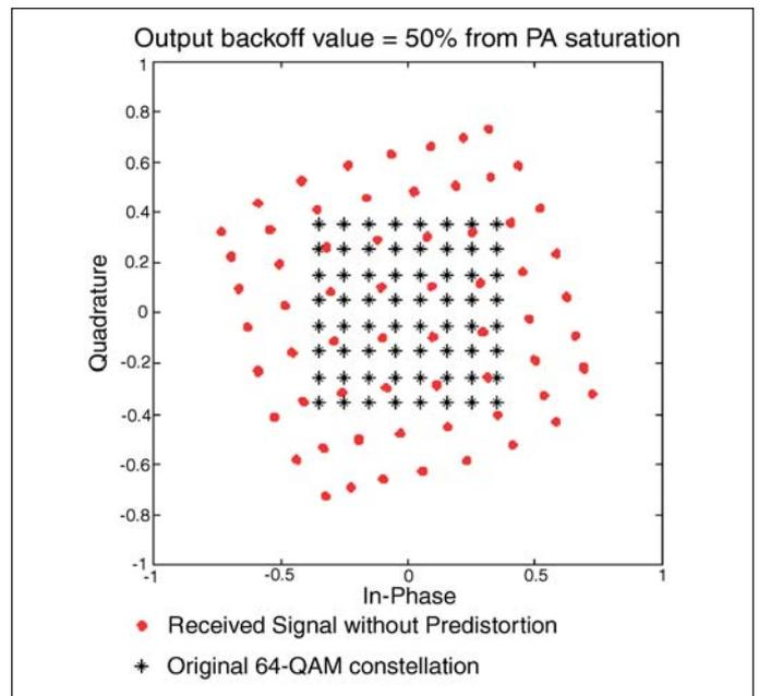
Figure 5 · Constellation warping due to nonlinear PA response in the absence of predistortion.
