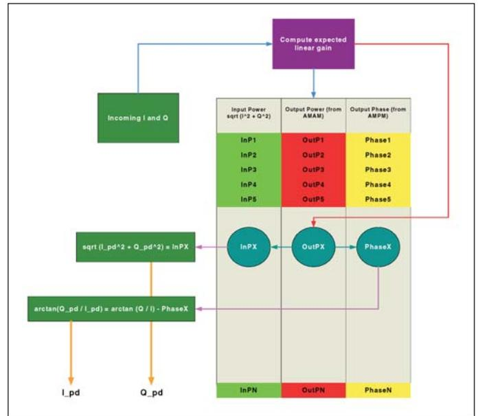
Figure 4 · Overall predistortion algorithm and LUT structure, where column one represents the input power, column two the resulting output power and column three the resulting output phase.
