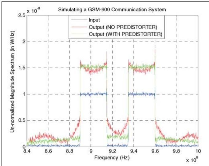
**Figure 10** . Simulating predistortion for a GSM-900 communication system.
