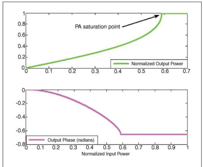
**Figure 9 · Amplitude and phase characteristics of the predistorter block.**
