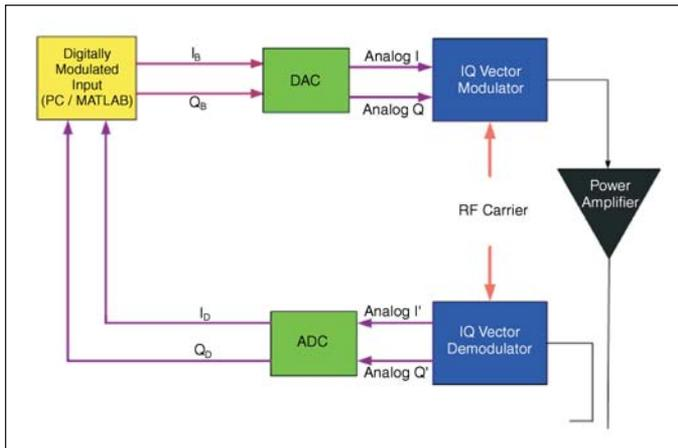
Figure 3 · Functional block diagram of the proposed digital baseband PA predistorter.
