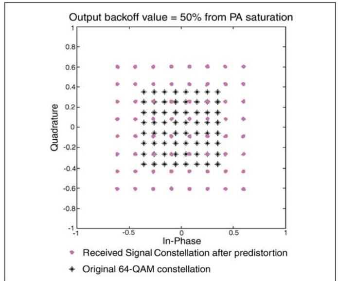
**Figure 7 · Nearly linear scaling of the transmitted constellation after predistortion.**
