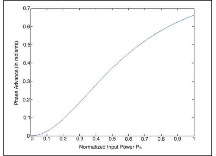
Figure 2 · Normalized phase response of PA as a function of normalized input power.
