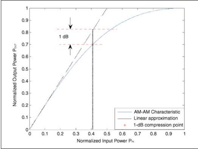
Figure 1 · Normalized output response of PA as a function of normalized input power.
