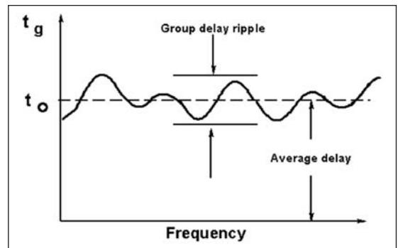
Figure 19 · Group delay ripple indicates a time-versus-frequency distortion.
