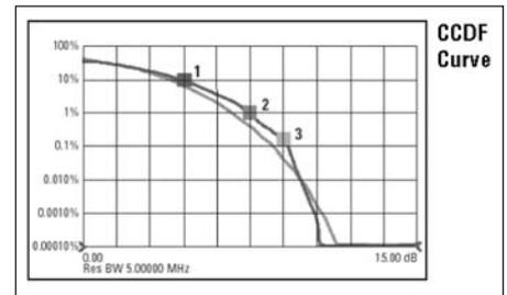
Figure 24 · Complementary cumulative distribution function of a RF waveform.
