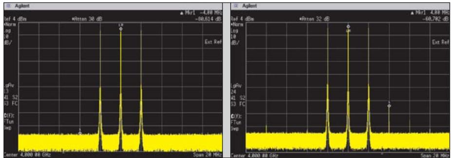
Figure 25 · Effect of power level on distortion.
