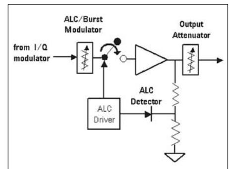
Figure 26 · Automatic level control circuit.
