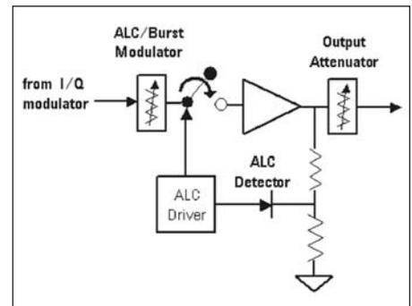
Figure 26 · Automatic level control circuit.
