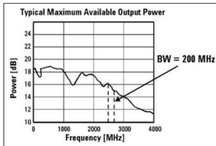
Figure 29 · Pass band ripple and roll-off of a signal generator.
