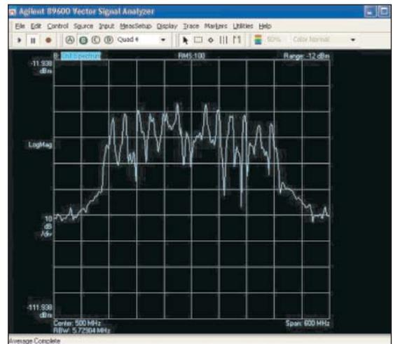
Figure 20 · 400 MHz bandwidth OFDM waveform spectrum.
