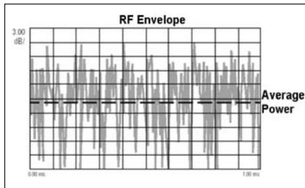
Figure 23 · Power envelope of an RF waveform.
