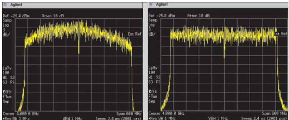
Figure 32 · Effect of predistortion on the flatness of a UWB signal.
