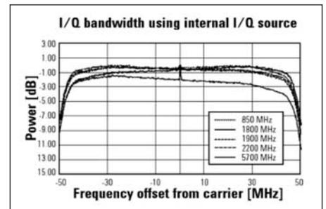
Figure 30 · Agilent ESG baseband bandwidth.
