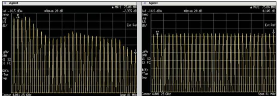
Figure 31 · Effect of predistortion on amplitude flatness.
