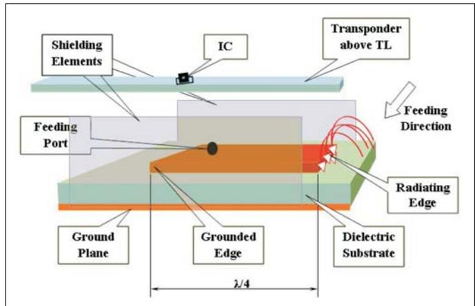
Figure 6 · Open Transmission Line antenna— $\lambda/4$  wavelength microstrip patch.
