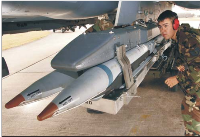
A bomb rack unit carrying four Small Diameter Bombs is loaded onto an F-15E Strike Eagle at Royal Air Force Lakenheath, England. (U.S. Air Force photo/Master Sgt. Lance Cheung)
