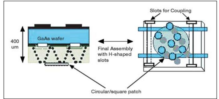
Figure 6 . Active antenna design using slot coupling to the GaAs wafer.
