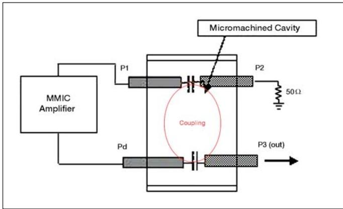
Figure 2 · Concept of slot coupling in GaAs wafer.
