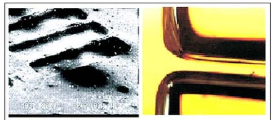
Figure 1 · Micromachining examples on GaAs wafer.
