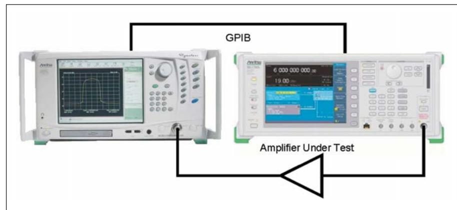
Figure 1 · ACPR Measurement Setup.
