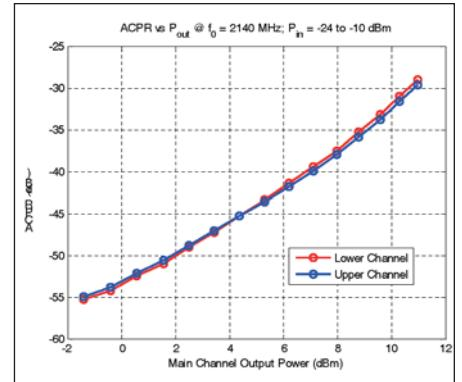
Figure 2 · ACPR vs. output power plot of a Mini-Circuits ZEL-1724LN generated by ACPRvsP.m.
