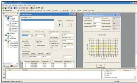
providing easy setup of signal simulation scenarios for testing EW radar, Elint systems and other receivers. The photo shows the AX user interface for a typical radar scan signal simulation using the list mode editor.
