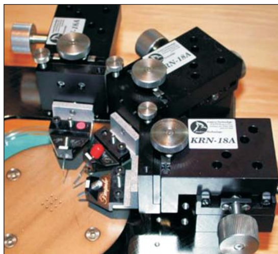
Figure 1 · Probes for microwave device measurements, mounted in adjustable probe holders (1).
