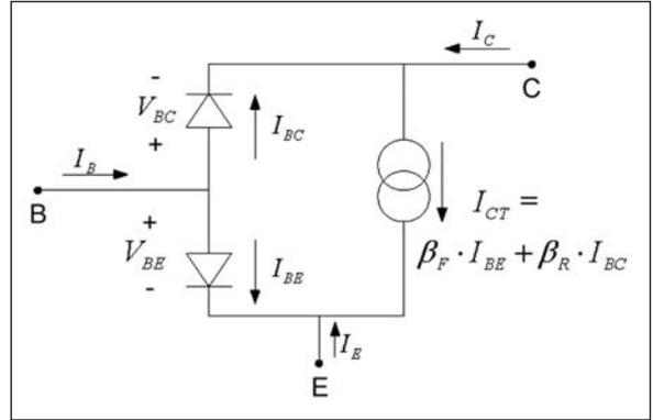
Figure 6 · The non-linear hybrid- $\pi$  version of the EM1 model.
