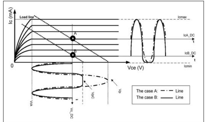
**Figure 4 · Idealized voltage—current waveforms at the output of an ideal BJT/HBT.**
