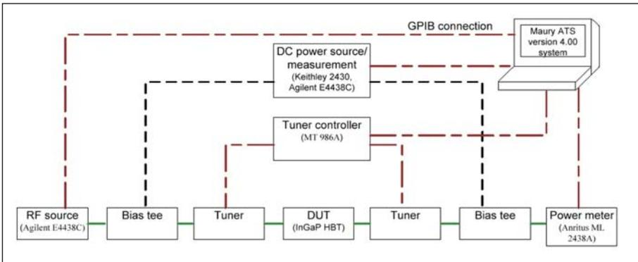
Figure 2 · Test configuration for power sweep measurements. (Tuners set to 50Ω condition for the results presented.)
