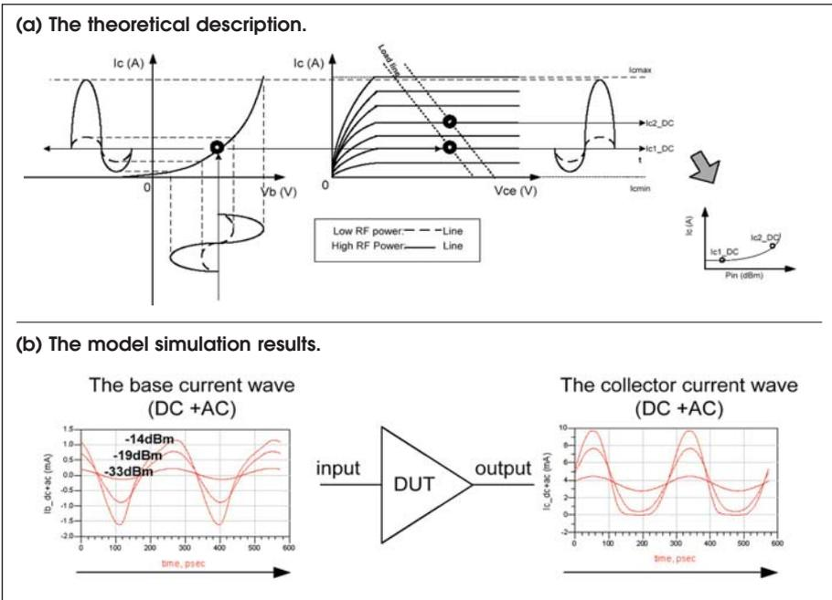
Figure 9 · Input voltage and output current waveform with a constant base voltage.
