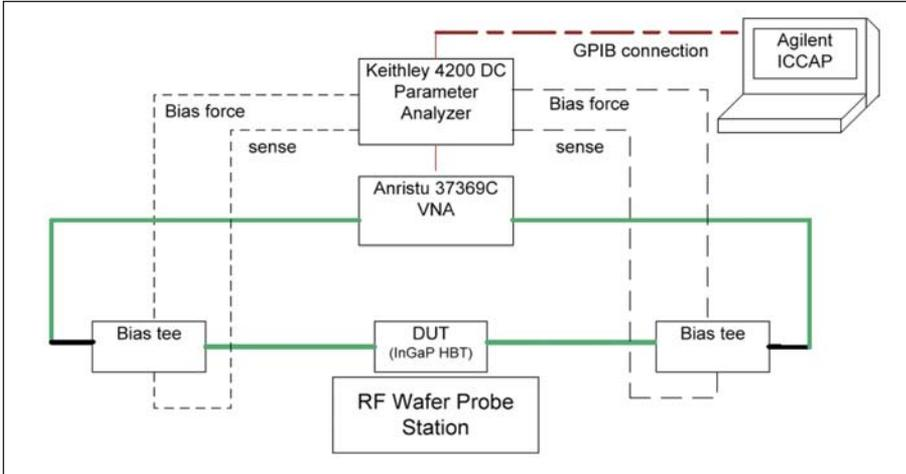
Figure 1 · DC/RF parameter test configuration for transistor model development.
