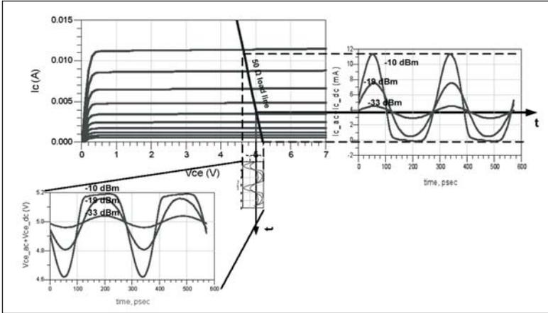
Figure 5 · Simulation showing the AC collector current and voltage waveform with various input RF power levels.
