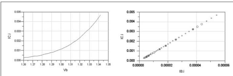
Figure 7 · The simulation of the  $I_c$  vs  $V_b$  and the  $I_c$  vs.  $I_b$  for the example InGaP/GaAs HBT (with self-heating effects deactivated).
