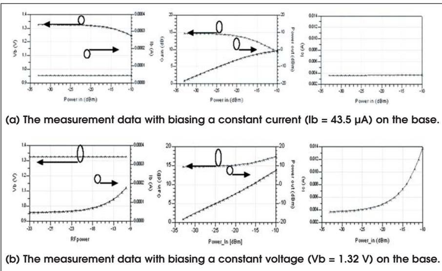
Figure 3 · The 50 ohm power sweep measurements of the InGaP HBT with different constant bias condition on the base with the RF frequency, 3.5 GHz and the bias condition  $V_{ce} = 5\text{ V}$  and  $I_c = 3.6\text{ mA}$ .
