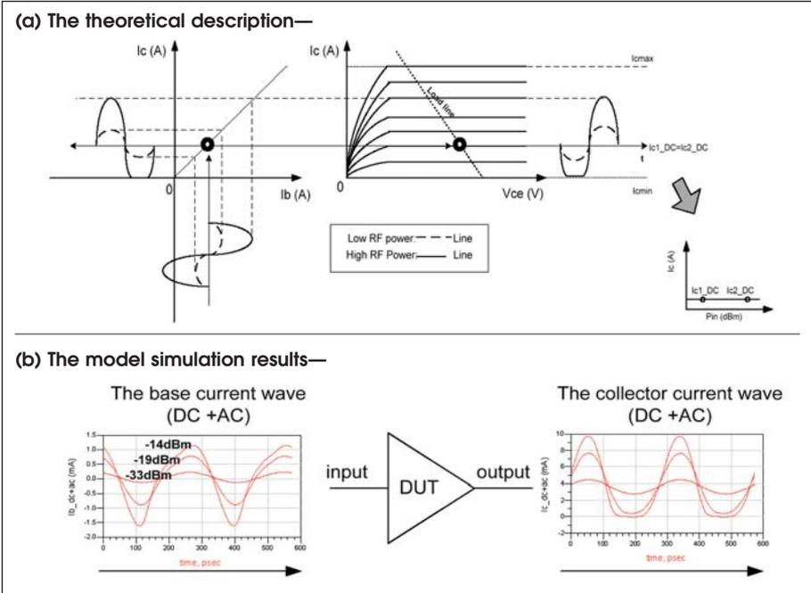
Figure 8 · The input current and output current waveform with a constant base current.
