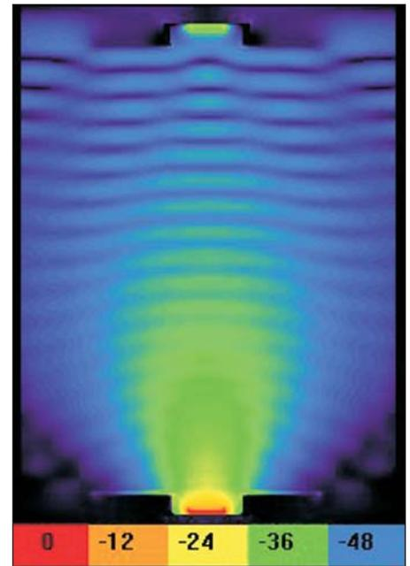
Figure 6 · Electromagnetic fields of a vertical cut near center; 2.4 GHz couplers on a 51 cm concrete wall.
