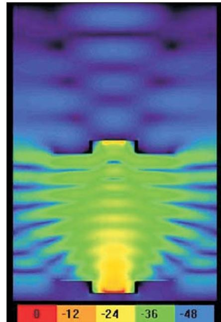
Figure 4 · Electromagnetic field of a vertical cut for 2.4 GHz couplers on a 25 cm concrete wall.
