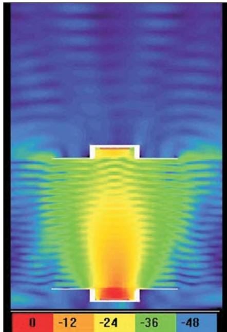
Figure 3 · Electromagnetic field of a vertical cut for 5.3 GHz couplers on a 25 cm concrete wall.
