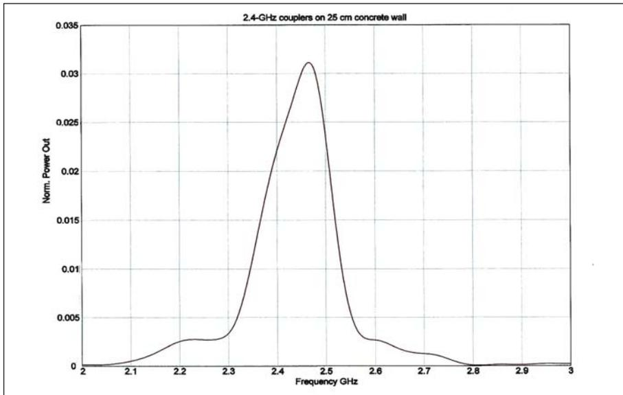
Figure 5 · Normalized output power of the receiving 2.4 GHz coupler communicating through a 25 cm concrete wall.
