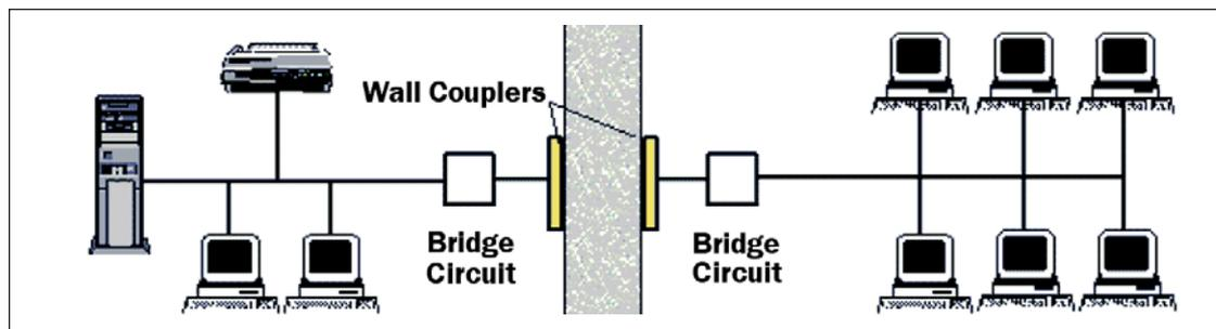
Figure 1 · Through-wall couplers eliminate the need for repeaters or wired connections.
