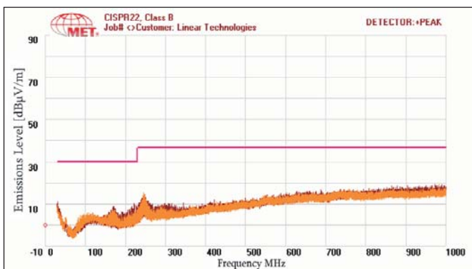
Figure 3b · LTM8032 emissions for 20 watts out, 36V IN .
