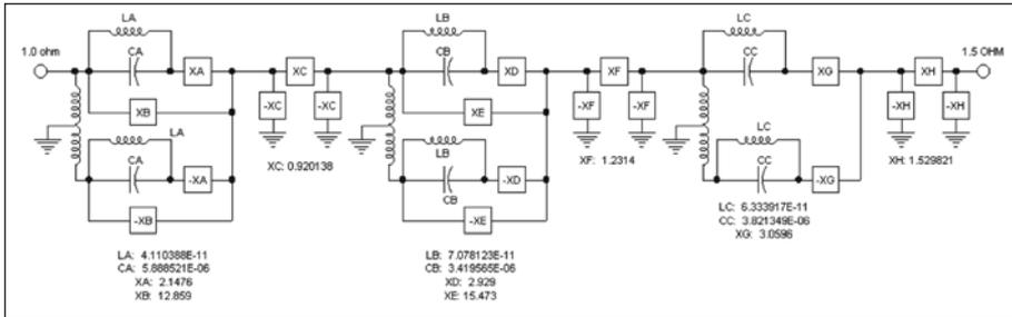
Figure 7 · Initial results of the bandstop transform.
