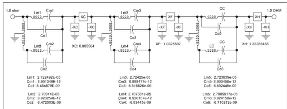
Figure 10 · The network after equalizing the inductor values.
