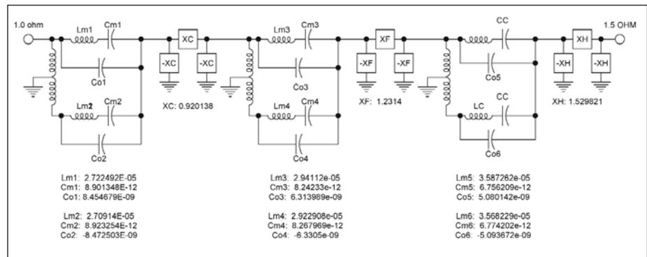
Figure 9 · Bandstop network after simplification.
