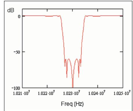
Figure 8 · Bandstop filter frequency response.
