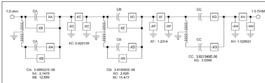
Figure 5 · Lowpass to high-pass transform.
