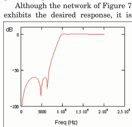
Figure 6 · Frequency response after highpass transformation.
