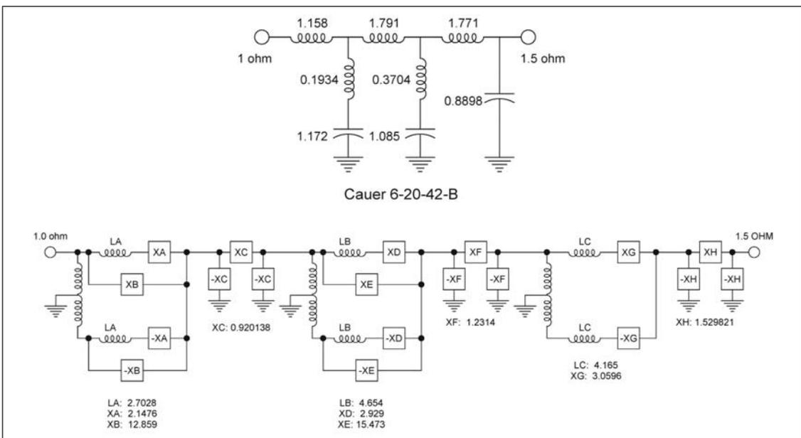
Figure 1 · Holt and Gray lowpass transform (bottom) from an elliptic lowpass prototype.
