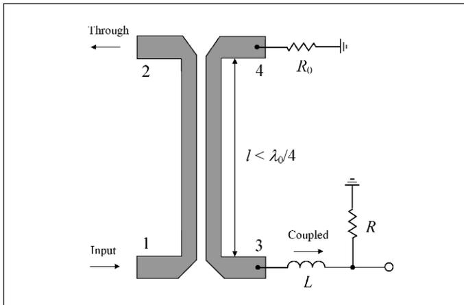
**Figure 43** . Coupled-line directional coupler with reduced-size and frequency compensation.
