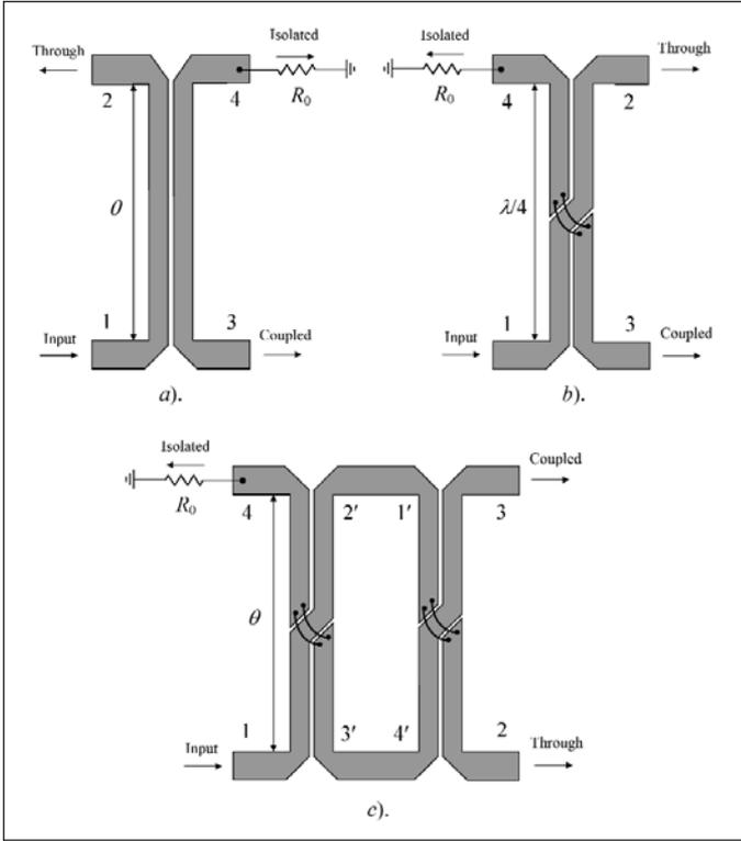
Figure 40 · Coupled-line directional couplers.
