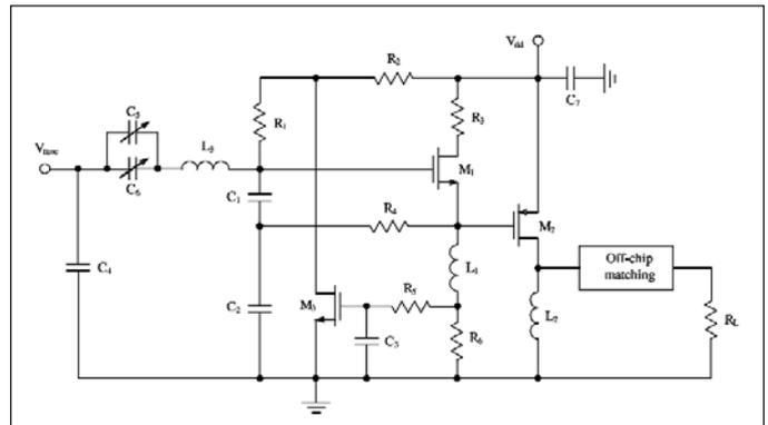
Figure 19 · CMOS VCO with low frequency feedback (21).
