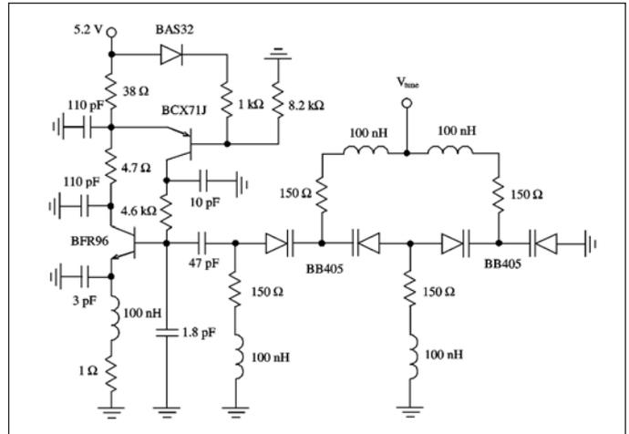
Figure 18 · Bipolar oscillator schematic with collector noise feedback (20).
