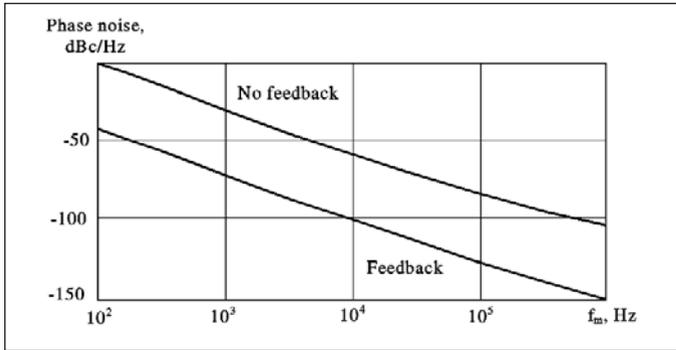
Figure 17 · Phase noise of bipolar oscillator with and without feedback.
