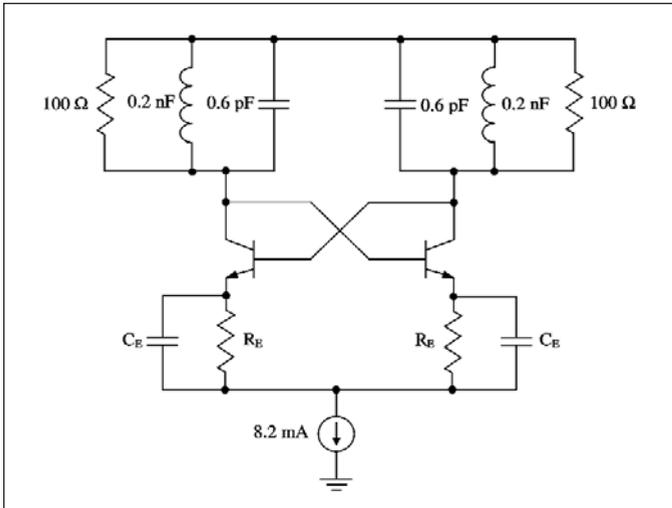
Figure 14 · VCO topology incorporating emitter degeneration.
