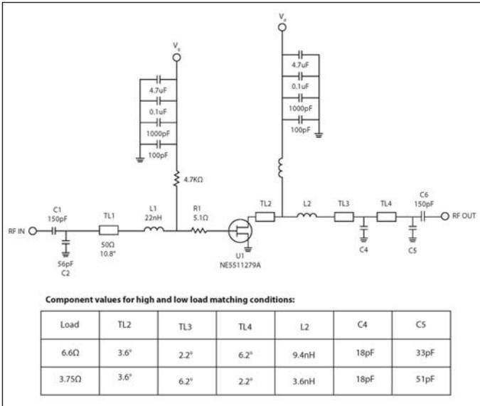
Figure 6 · Schematic of circuits for two additional load conditions.
