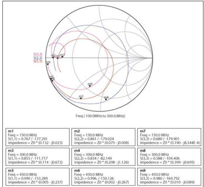
Figure 7 · Smith chart plots for three load impedances up to 3rd harmonic frequency.
