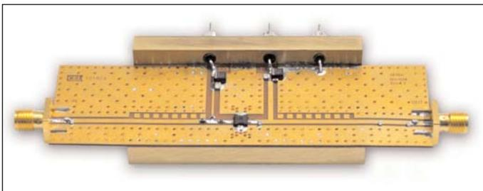
Figure 3 · Photo of the constructed PA circuit board.
