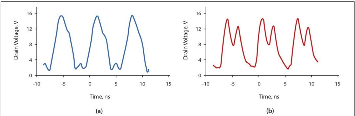
Figure 14 · Measured waveforms of: (a) high efficiency circuit and (b) high power circuit.
