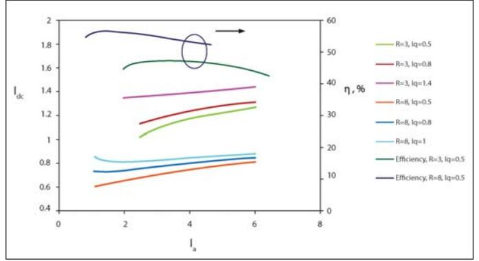
Figure 12 ·  $I_{dc}$  vs  $I_a$  from numerical analysis of the saturation model at two load conditions of  $R = 3$  and  $8$ . The starting points of  $I_a$  are different because the region where the model is valid varies.
