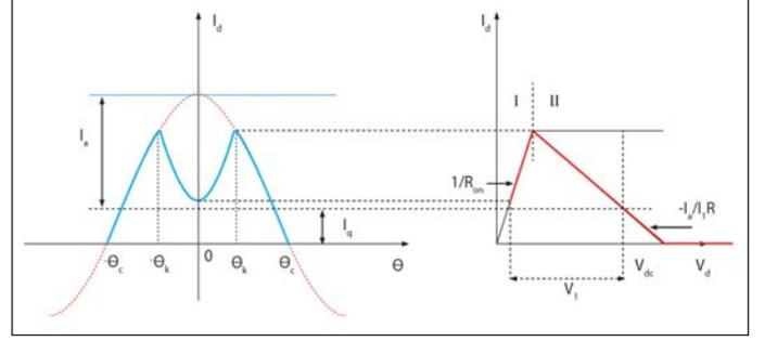
**Figure 11 · Drain current saturation model.** The left is the waveform derived from the ideal I-V curve on the right and Eq. 4-6. The parameters are:  $I_a = 3$ ;  $I_q = 1$ ;  $V_{dc} = 7.5$  V;  $R_{on} = 1\Omega$ ;  $R = 5\Omega$ . The red line on the right is the trajectory in the  $(I_d, V_d)$  plane for one RF cycle.
