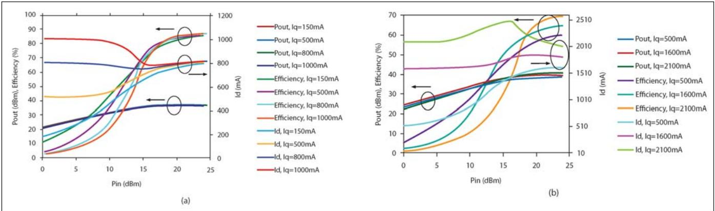
Figure 9 · Dependence of output power, efficiency and drain current with input power. (a) high efficiency load; (b) high power load.
