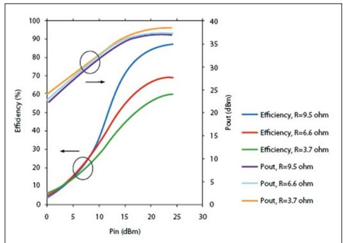
Figure 8 · Output power and efficiency vs. input power for three load conditions.
