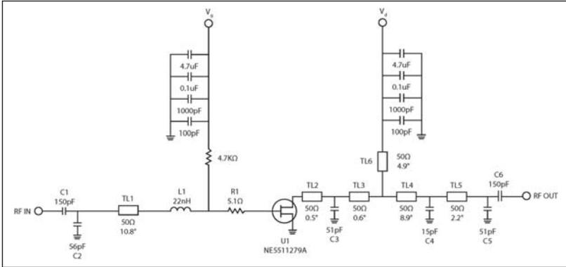
Figure 2 · Schematic of a high efficiency 5 W, 150 MHz power amplifier using NE5511279A.
