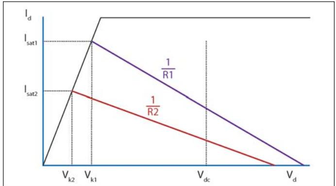
Figure 5 · Illustration of the effect of load line on efficiency.  $R_1 < R_2$ .
