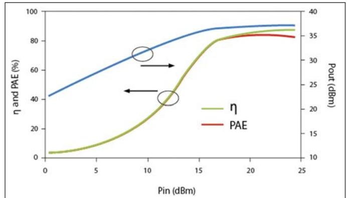
Figure 4 · Output power,  $P_{out}$ , drain efficiency,  $\eta$  and power added efficiency, PAE, versus input power,  $P_{in}$ , drain voltage,  $V_d = 7.5$  V, quiescent current,  $I_q = 800$  mA.
