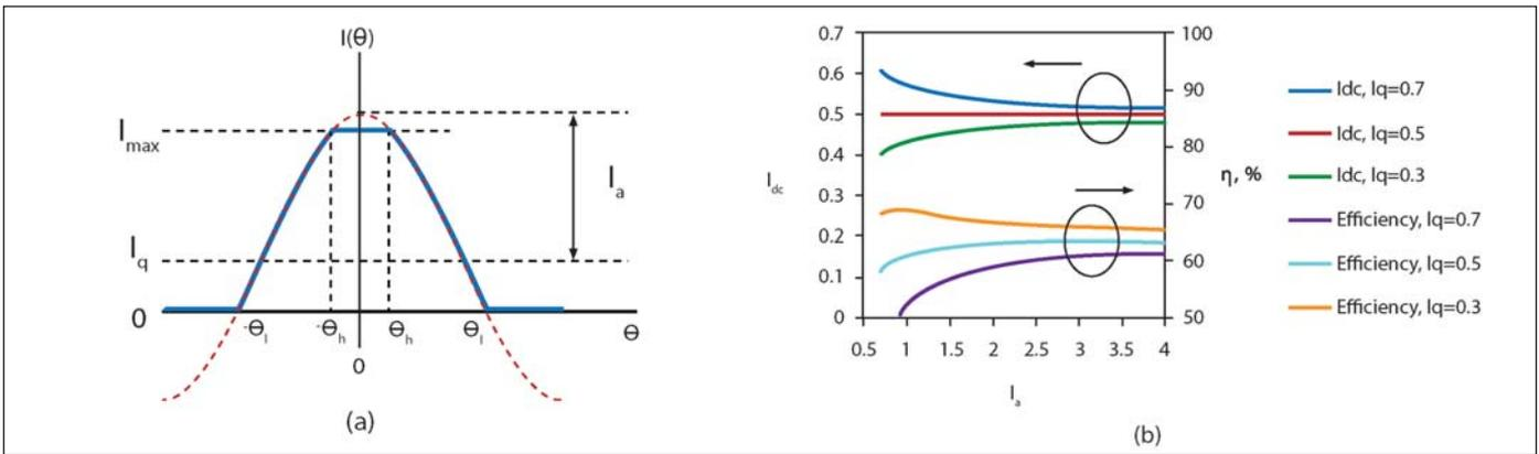
Figure 10 · Clipping effect. (a) Dashed line: undistorted waveform, sine wave plus DC; Solid line: the waveform is limited to the range  $(0, I_{max})$ ; (b) DC component,  $I_{dc}$  and efficiency,  $\eta$  of the waveform in (a) as a function of amplitude,  $I_a$  for three  $I_q$  values.  $I_{max}$  is normalized to 1.
