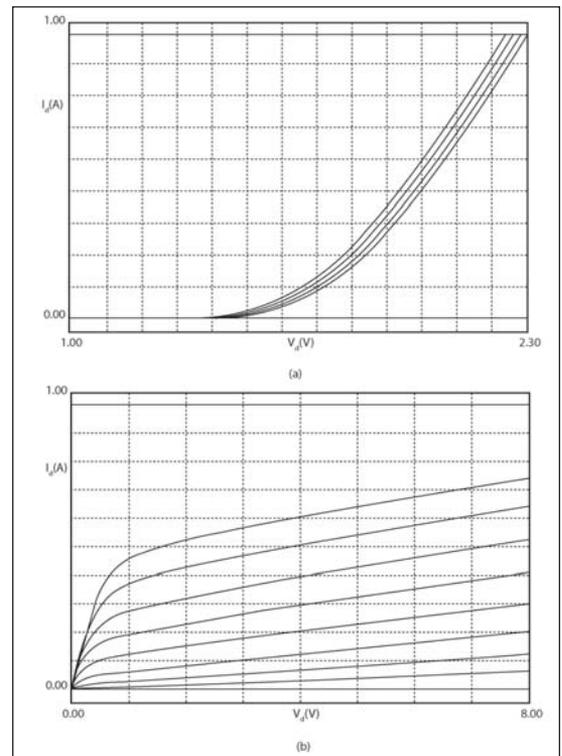
Figure 1 · DC characteristics of the Renesas NE5511279A: (a) Transfer curves; (b) I-V curves.
