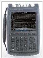
er includes these functions: spectrum analyzer, power meter with USB power sensor, and a vector network analyzer option. The unit can make the necessary insertion gain/loss, VSWR and distance-to-fault measurement common in wireless system installation and maintenance. A key feature of the FieldFox is QuickCal, a built-in calibration system that does not require a calibration kit.
