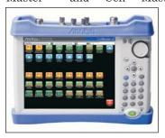
S331E/S332E/S361E/ S362E are full-featured handheld analyzers for installing, provisioning, maintaining, and troubleshooting wireless base station cable and antenna systems. The MS2712E/MS2713E handheld spectrum ana-
