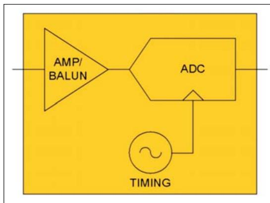
Figure 1 · Block diagram of a data capture and conversion core.
