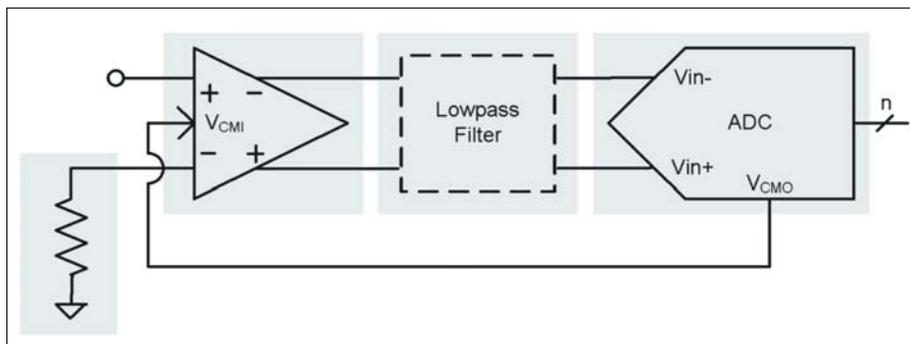
Figure 4 · Amplifier in DC-coupled configuration.
