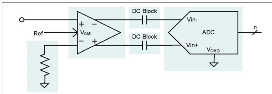
Figure 5 · Amplifier in AC-coupled configuration.
