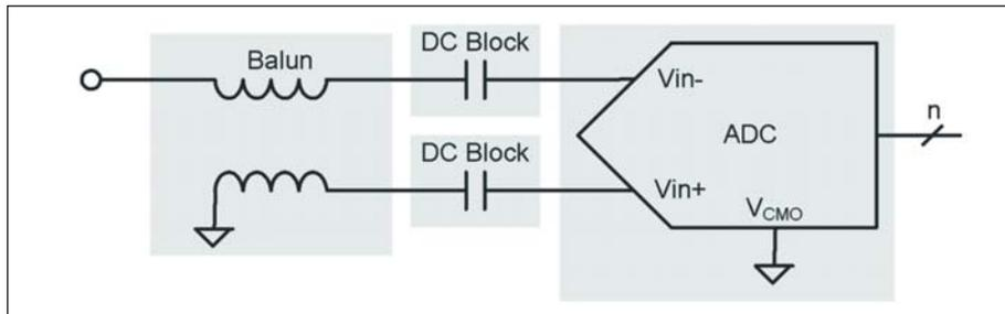
Figure 3 · Balun in AC-coupled configuration.
