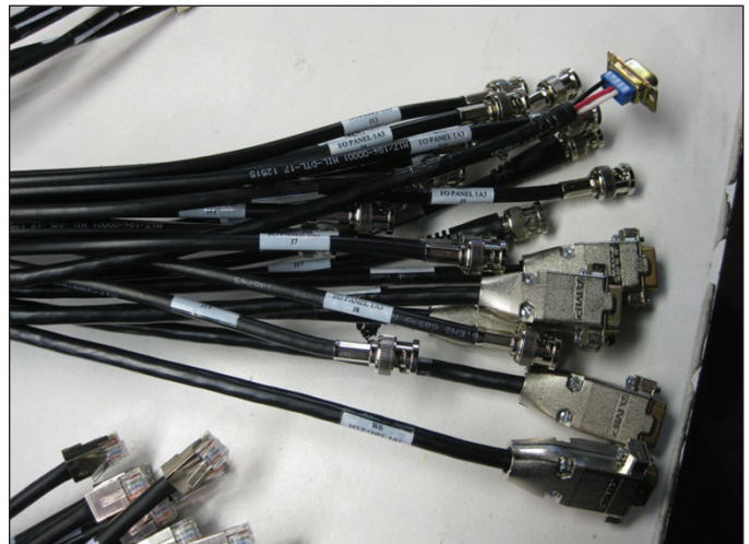
Figure 4 • Thirteen different types of connectors were used for each assembly.
