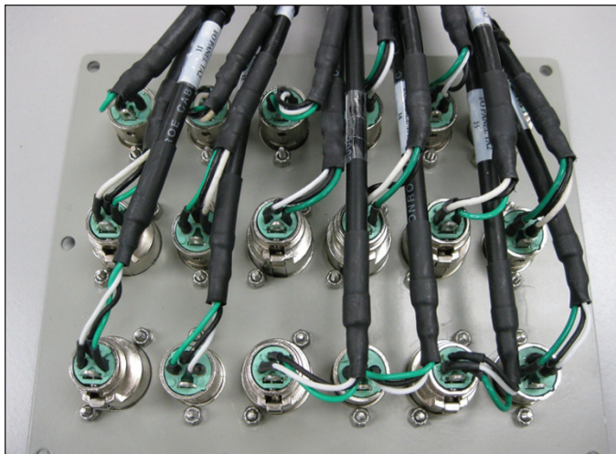
Figure 1 • A robust feed-through panel was vital for the vertical orientation of the installation.
