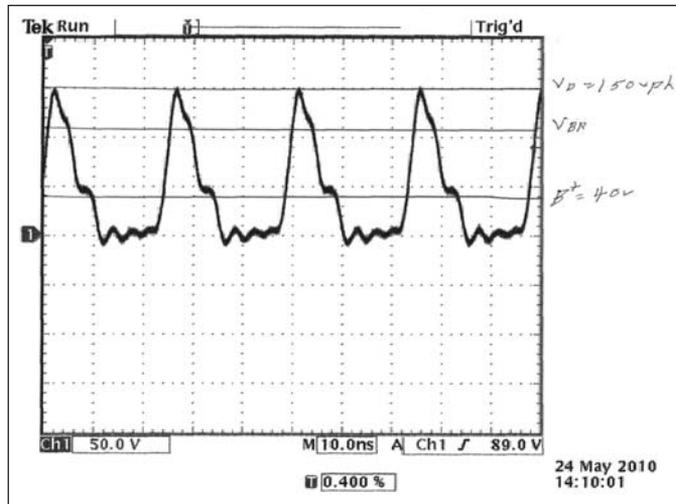
Figure 1 · Drain voltage waveform:  $P_v = 544$  W; Eff. = 85%; 40.68 MHz.
