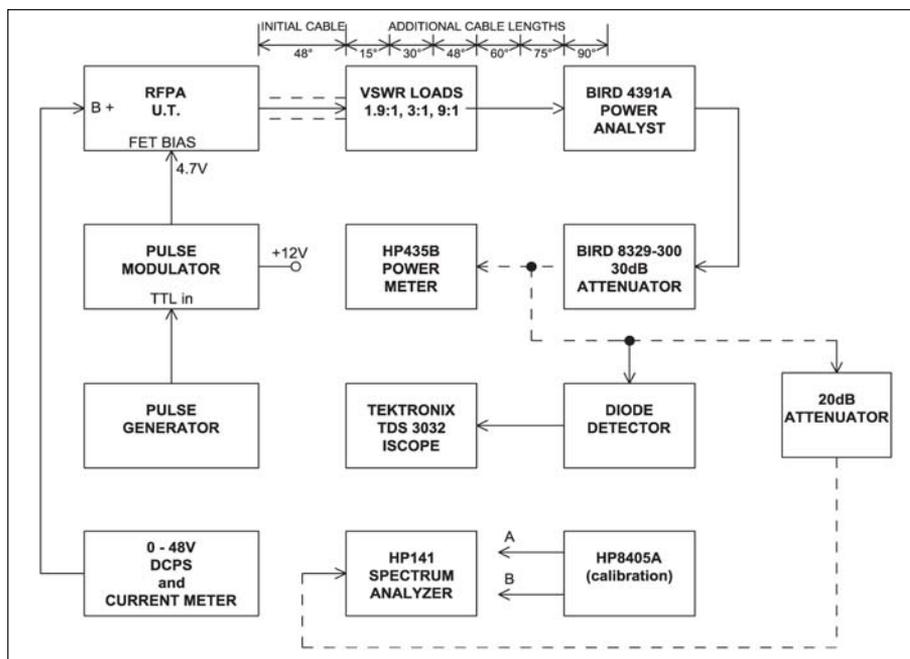
Figure A1 · RFPAs VSWR testing block diagram.
