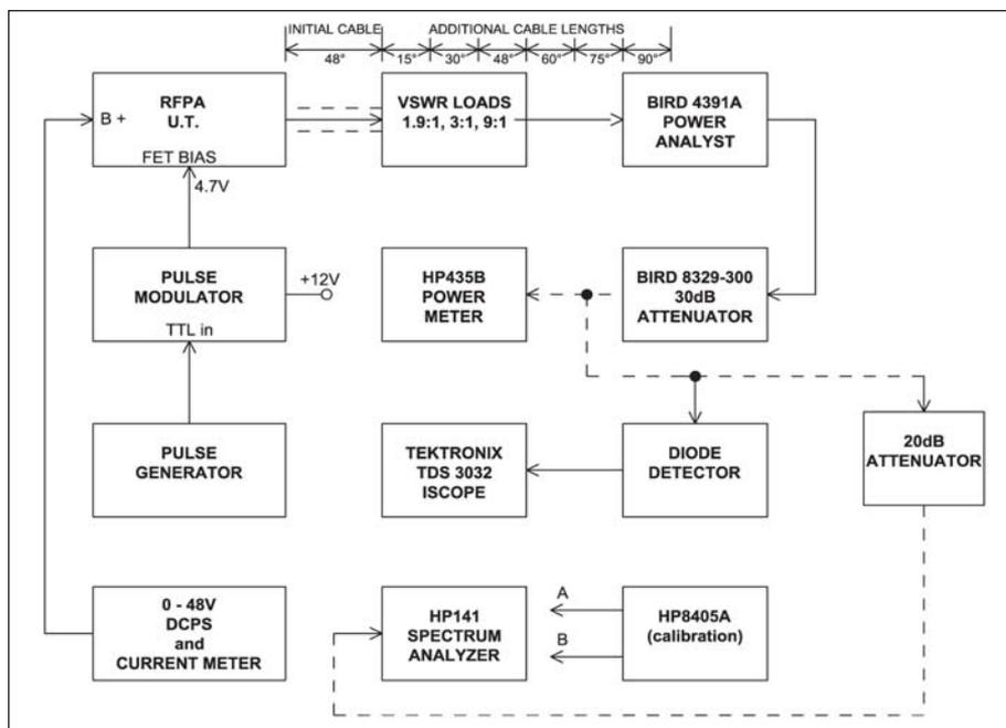
Figure A1 · RFPA VSWR testing block diagram.
