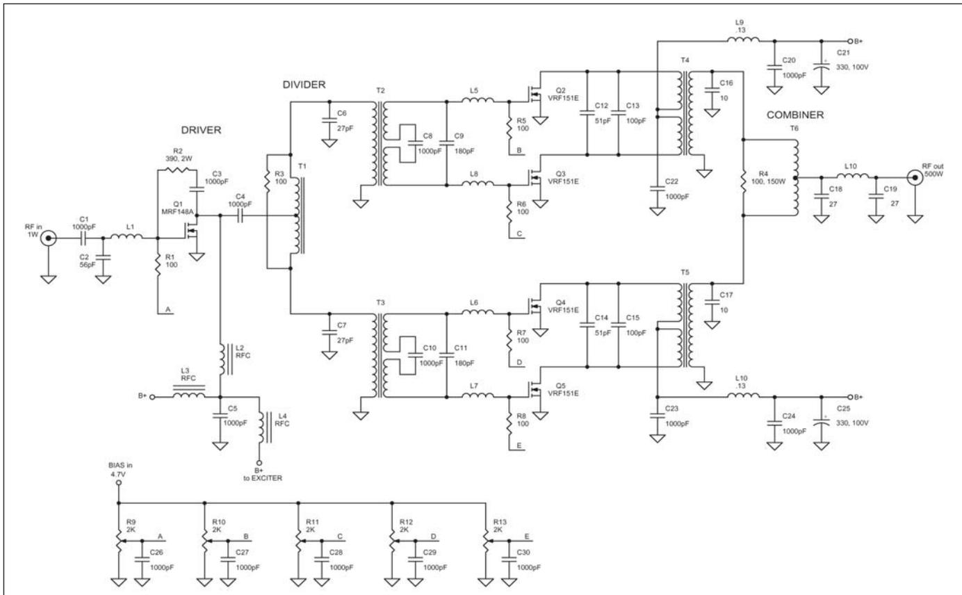
Figure A2 · RF power amp—81.36 MHz.
