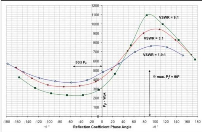
Figure A3 · Forward Power vs.  $\theta$  for VSWRs of 1.9:1, 3:1, 9:1.
