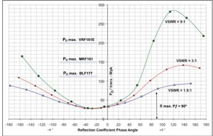
Figure A4 · Power dissipated per transistor vs.  $\theta$  for VSWRs of 1.9:1, 3:1, 9:1.
