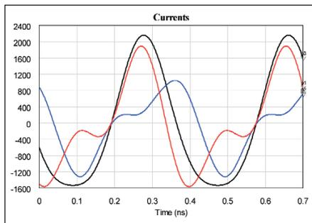
Figure 10 · Simulation of currents at Doherty output combiner node, single-tone  $P_{out} = 48$  dBm; black = output arm, red = carrier arm, blue = peaking arm.
