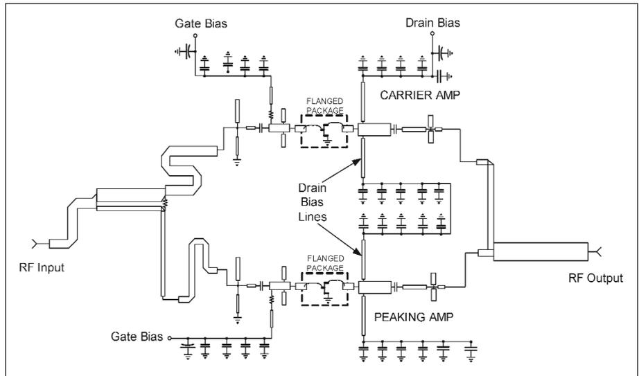
**Figure 5 · Doherty amplifier schematic.**
