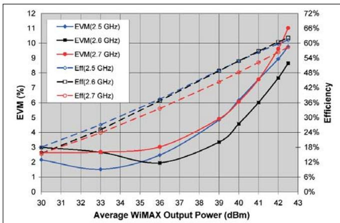
Figure 12 · Measured Doherty amplifier EVM and efficiency vs. WiMAX  $P_{out}$  (without predistortion).
