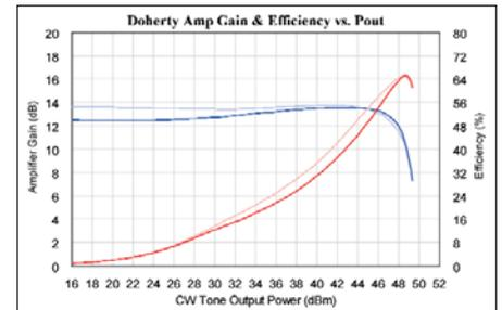
**Figure 3 · Simulated gain and efficiency vs. CW output power for two input couplers. Dark trace is for 3 dB (equal) coupling. Light trace is for approximately 1.8/4.7 dB coupling (more power to carrier amplifier versus peaking amplifier).**
