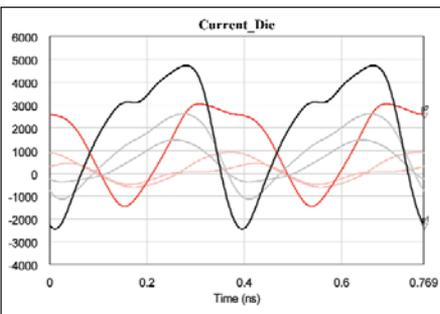
Figure 9 · Simulation of drain currents at the carrier (black) and peaking (red) transistors with single-tone  $P_{out} = 36, 42$  and 48 dBm.
