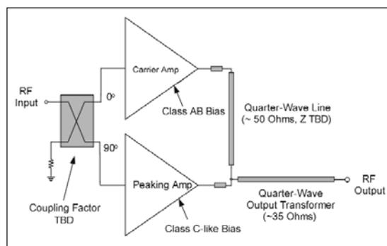
Figure 1 · A basic 2-way Doherty amplifier configuration.
