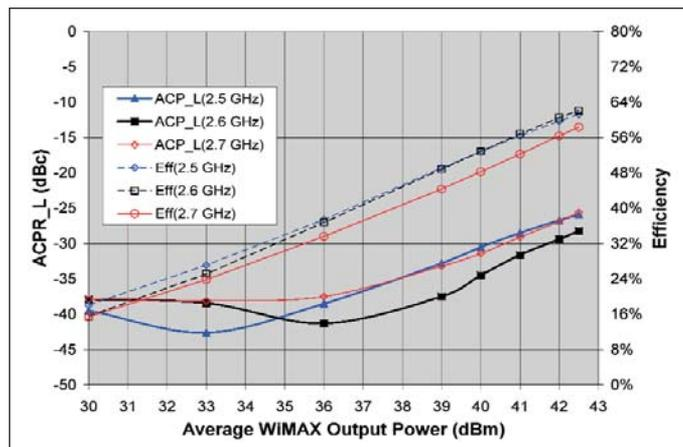
Figure 13 · Measured Doherty amplifier ACPR and efficiency vs. WiMAX  $P_{out}$  (without predistortion).
