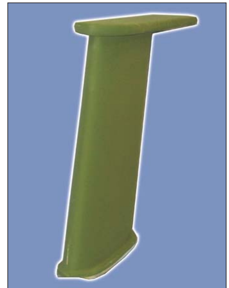
Figure 5 · Astron model AA-302000 Airborne Blade antenna, operating over 30 to 2000 MHz (readily extended to 2500 MHz), minimum gain of -10 dBi 30 MHz (over 5 dBi higher than available to date) with an average gain of over 0 dBi from 60 to 2000 MHz, 100 watts input power and a minimal VSWR of 2.5:1.
