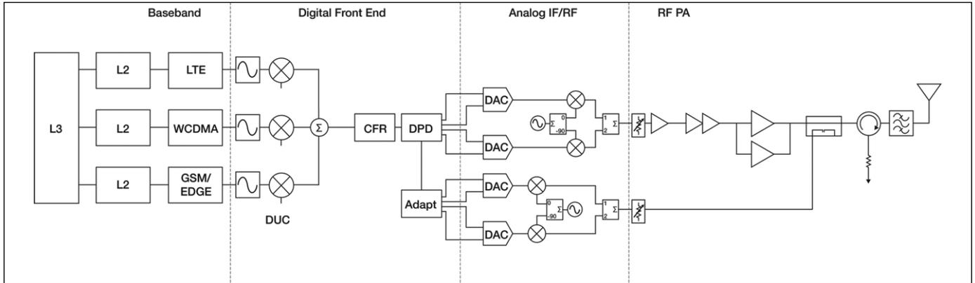
Figure 1 • A typical single-sector transmission link.
