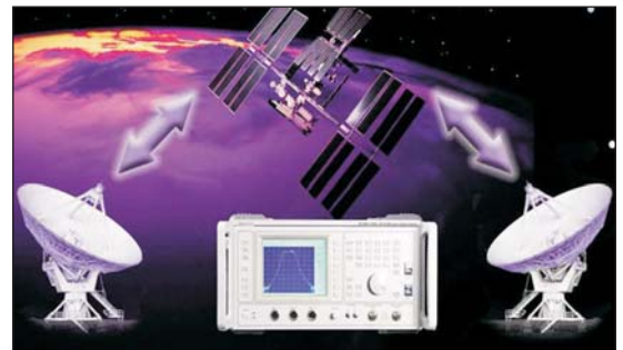
Figure 1 · To get the best performance out of a satellite link it is necessary to measure and accurately compensate for distortion caused by group delay at the band edges.
